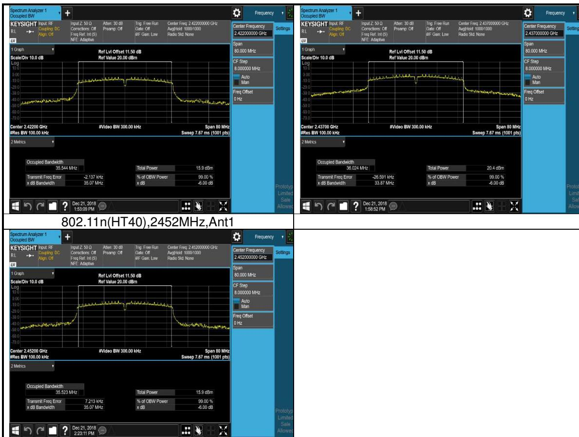
**TEST REPORT****3. Occupied Bandwidth****3.1 Test Data**
