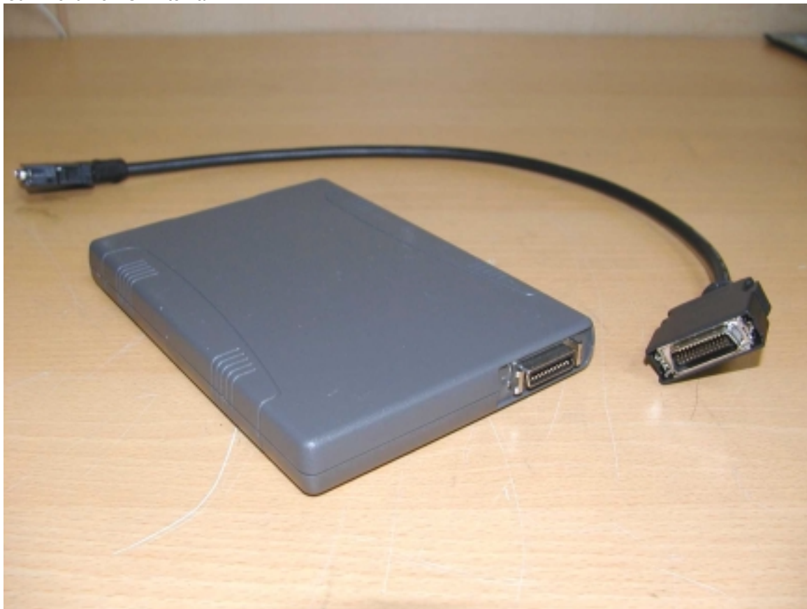
30. Front View Of External F.D.D.
