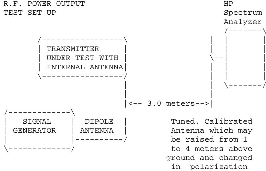
Equipment placed 80cm above ground on a rotatable platform.
