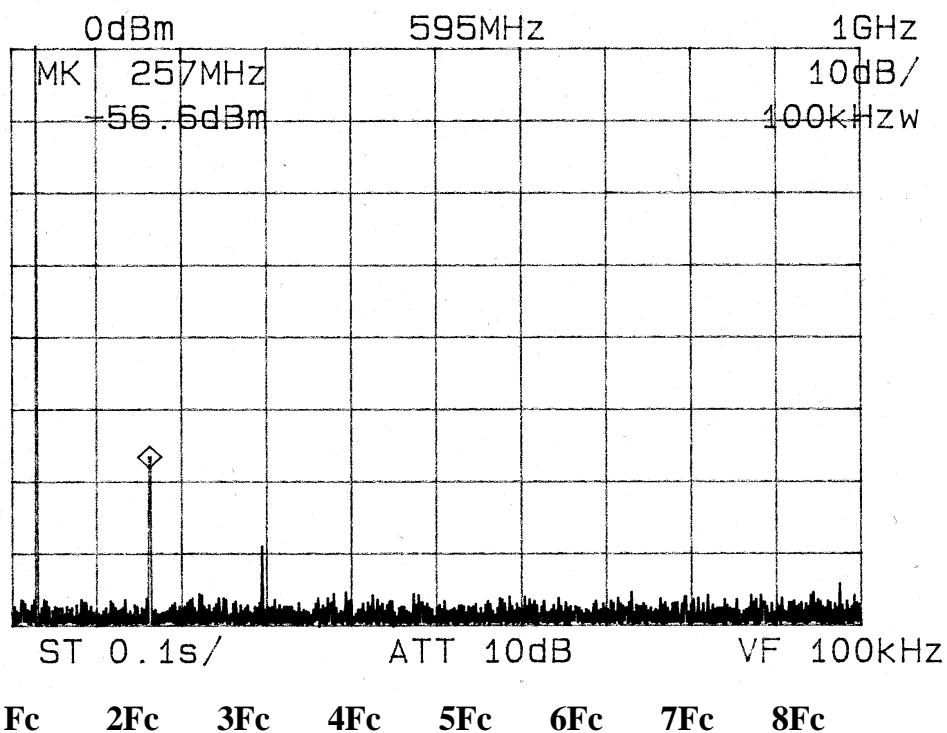
NOTE: 30 dB EXT. ATTN. / 1 GHZ SPAN / 100 KHZ RBW
