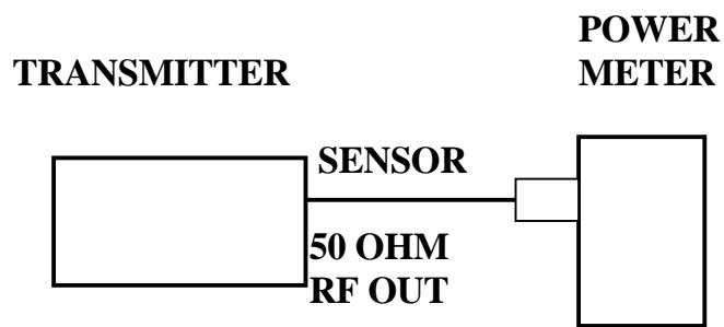
**RF Power Reading = 29.90 dBm @ 126.00 MHz**
