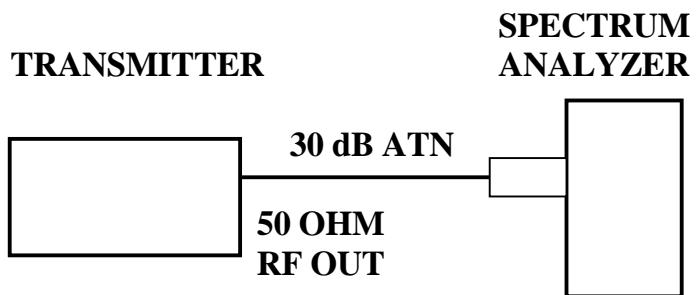
**CONDUCTED OUTPUT – UNMODULATED CARRIER @ 126.00 MHZ**
