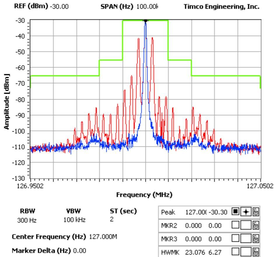
**SPURIOUS EMISSIONS AT ANTENNA TERMINALS (CONDUCTED)**
