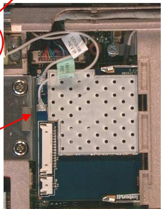
Inverted F antenna mounted on left side of LCD screen
