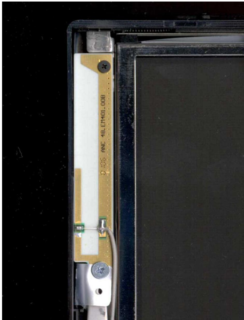
Slot antenna mounted on right side of LCD screen
