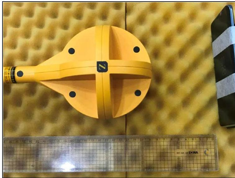
**Photo of MPE Test Set up at 13 cm distance (B-field)****Position A**
