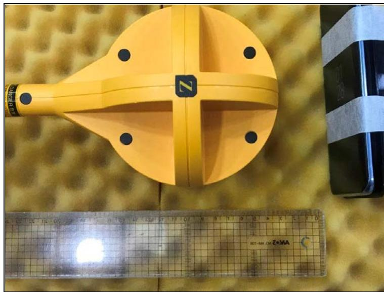
**Photo of MPE Test Set up at 8 cm distance (B-field)****Position A**
