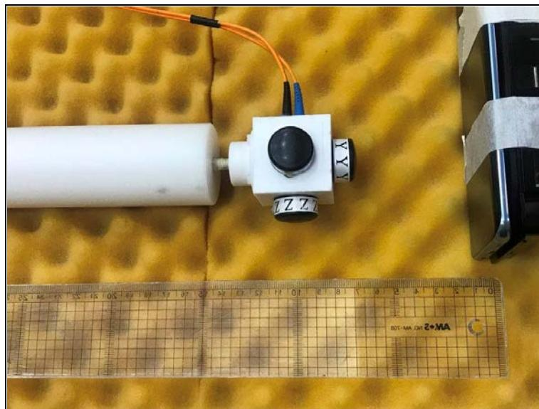
**Photo of MPE Test Set up at 8 cm distance (E-field)****Position A**
