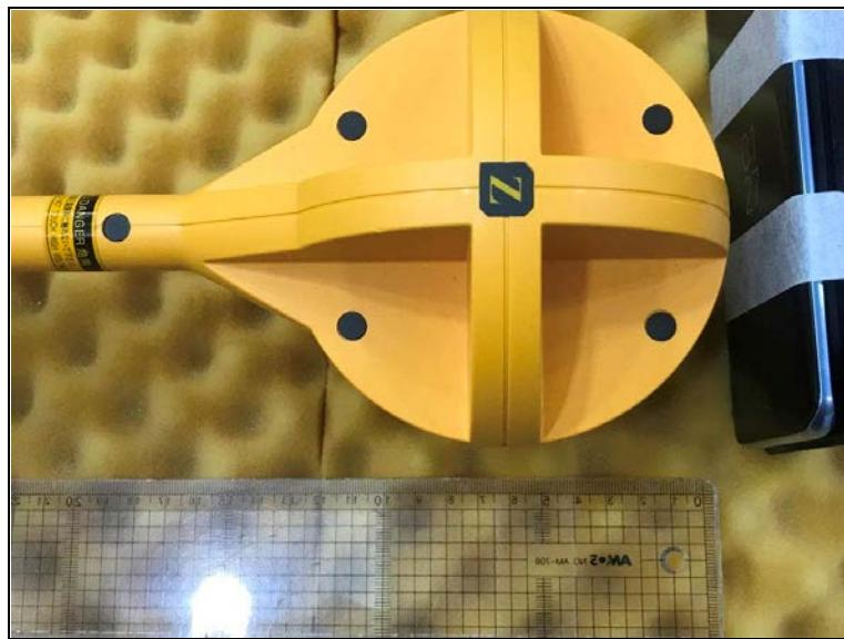
**Photo of MPE Test Set up at 15 cm distance (E-field)****Position A**
