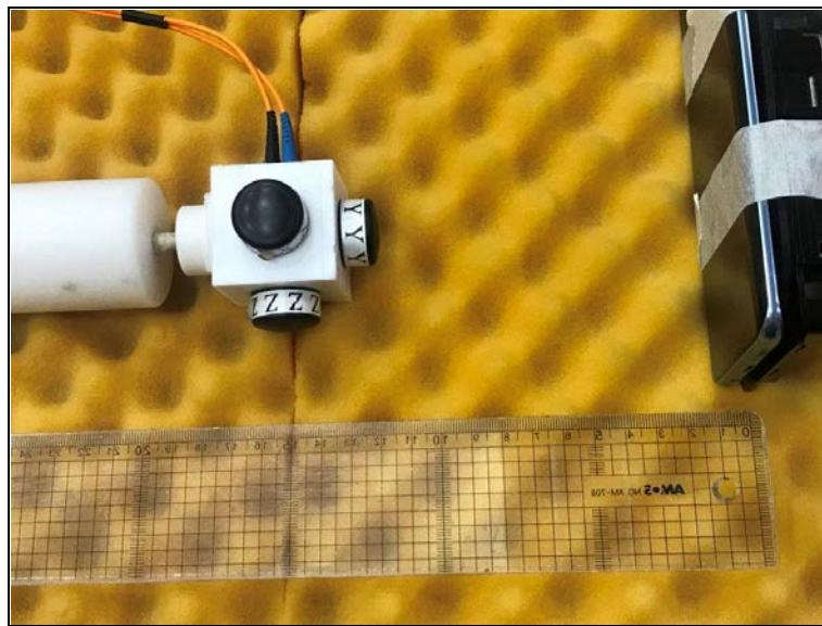
**Photo of MPE Test Set up at 13 cm distance (E-field)****Position A**
