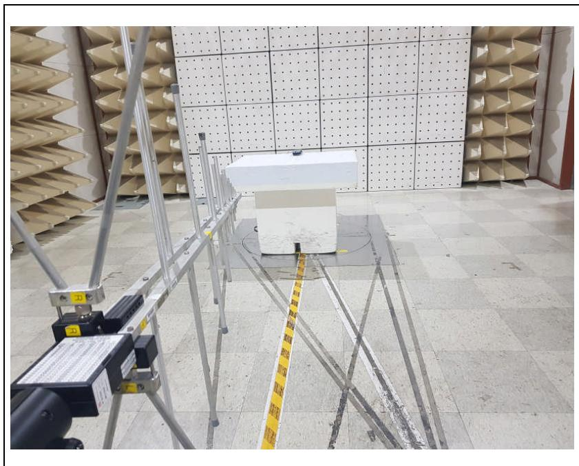
**Photo of MPE Test Set up at 15 cm distance (B-field)****Position A**
