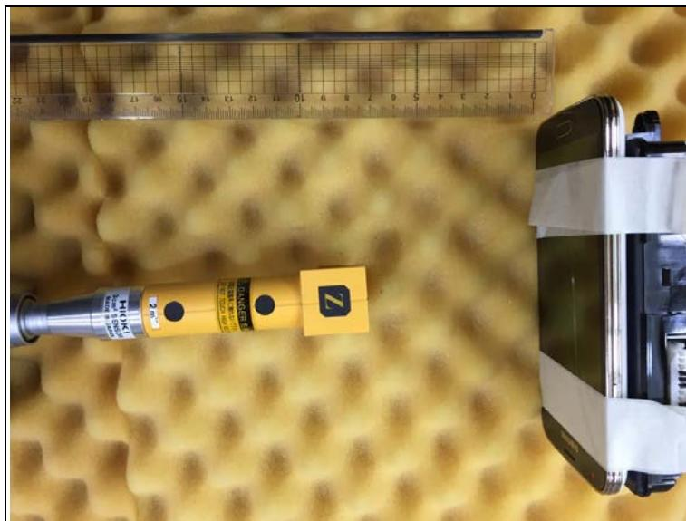
**Photo of MPE Test Set up at 6 cm distance (B-field)****Position A**
