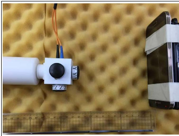
**Photo of MPE Test Set up at 13 cm distance (E-field)****Position A**
