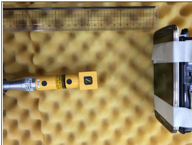
**Photo of MPE Test Set up at 8 cm distance (B-field)****Position A**
