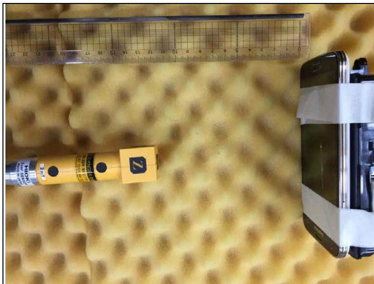
**Photo of MPE Test Set up at 10 cm distance (B-field)****Position A**
