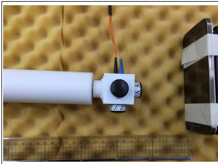
**Photo of MPE Test Set up at 8 cm distance (E-field)****Position A**
