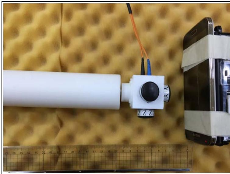
**Photo of MPE Test Set up at 4 cm distance (E-field)****Position A**
