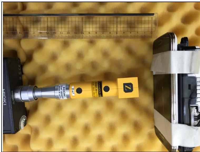
**Photo of MPE Test Set up at 15 cm distance (E-field)****Position A**
