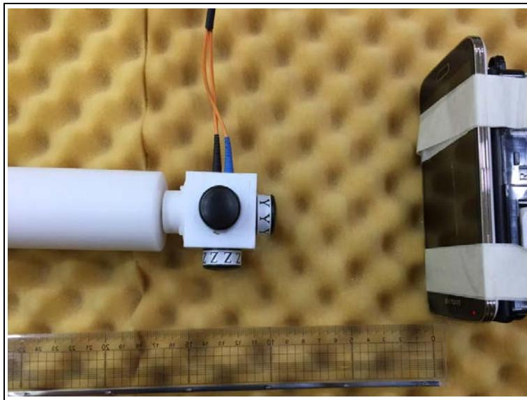
**Photo of MPE Test Set up at 10 cm distance (E-field)****Position A**
