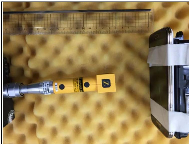
**Photo of MPE Test Set up at 4 cm distance (B-field)****Position A**
