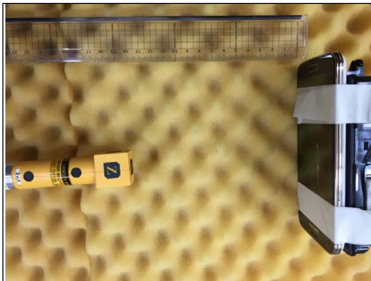
**Photo of MPE Test Set up at 13 cm distance (B-field)****Position A**
