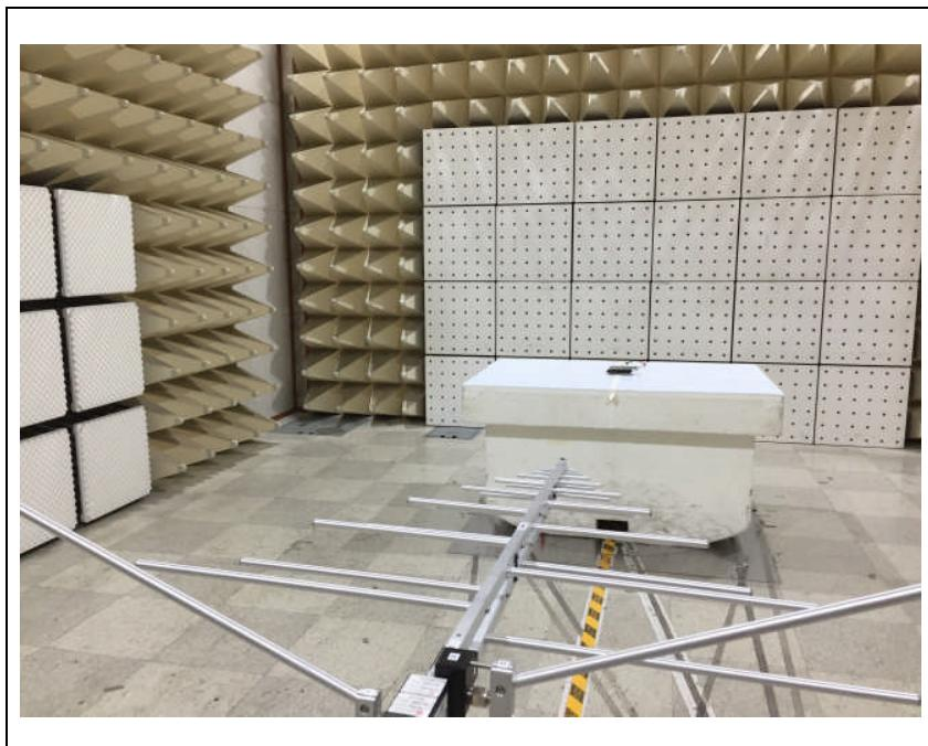
**Photo of MPE Test Set up at 15 cm distance (B-field)****Position A**
