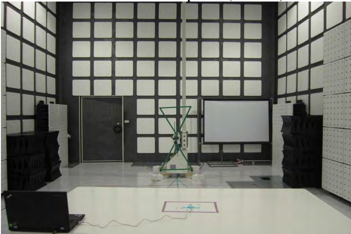
Radiated Emission Set up Photo (Below 1G)
