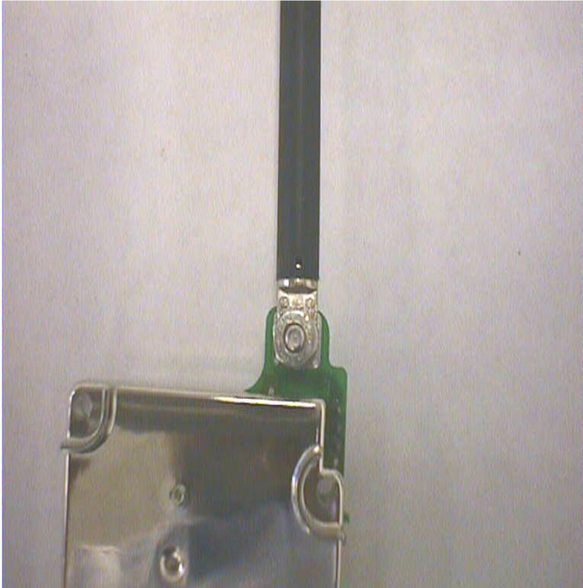
Ewave, Inc. Model: RF-10K Transceiver Internal product photo Fixed Internal Antenna
