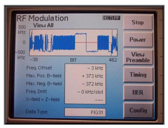
b) Carrier Frequency Stability over temperature
