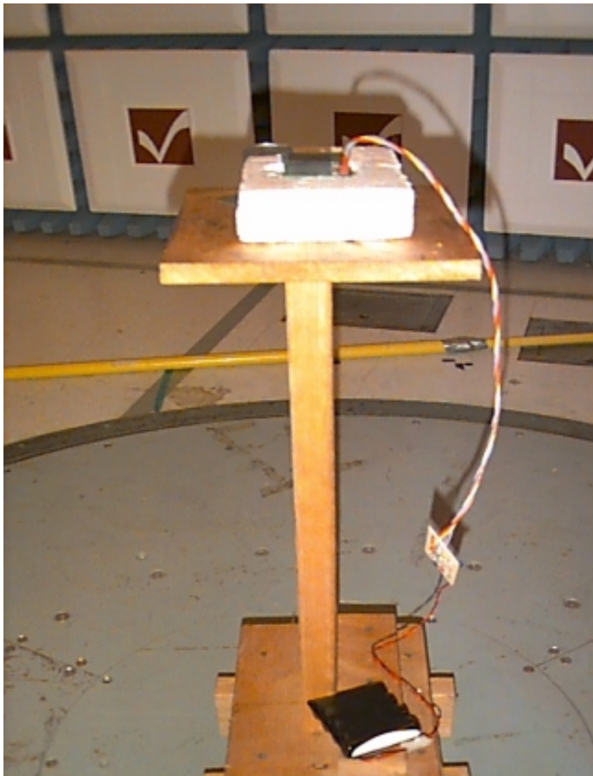
View of the T900 during the Radiated Emissions tests. This view shows the sample during the measurements above 5 GHz, while at the 1 meter range.
