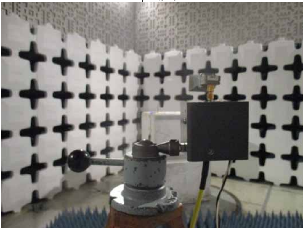
Test Setup for Radiated Emissions – 18GHz to 26.5GHz, Vertical Polarization Linx Whip Antenna
