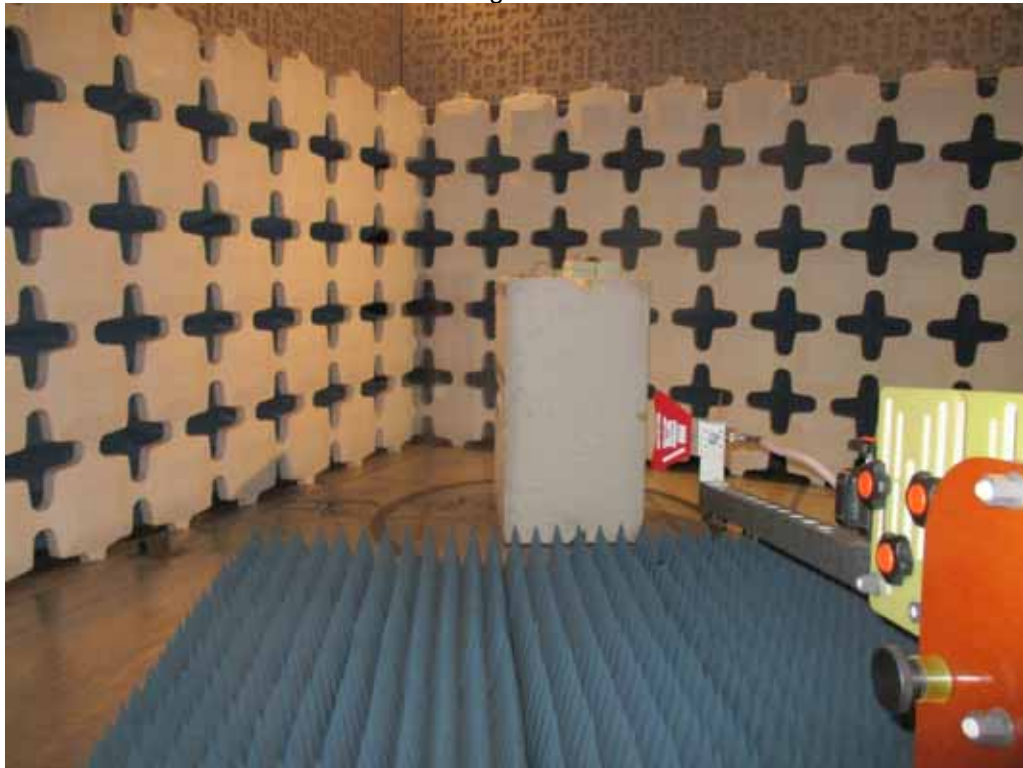
Test Setup for Radiated Emissions – 1GHz to 18GHz, Horizontal Polarization Taoglas Combo Antenna
