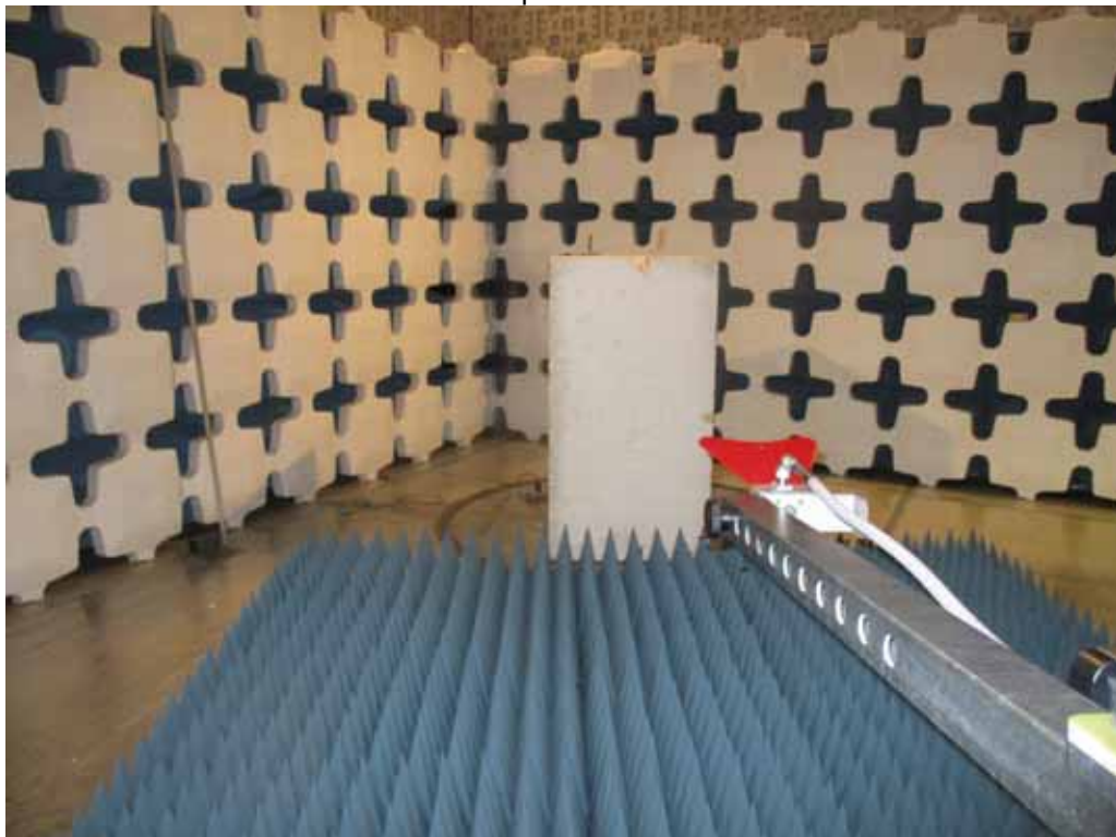
Test Setup for Radiated Emissions – 1GHz to 18GHz, Vertical Polarization Linx Whip Antenna
