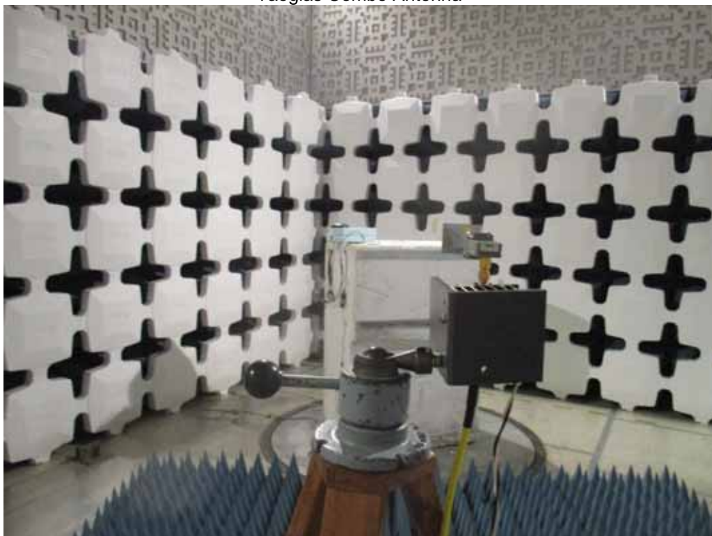
Test Setup for Radiated Emissions – 18GHz to 26.5GHz, Vertical Polarization Taoglas Combo Antenna
