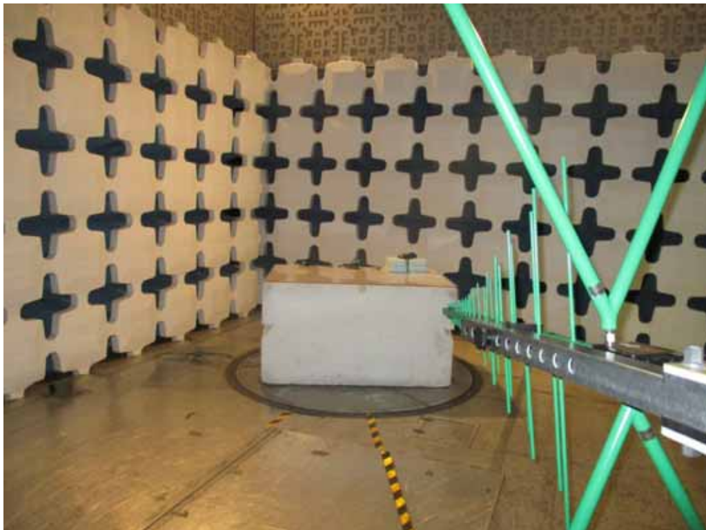
Test Setup for Radiated Emissions – 30MHz to 1GHz, Vertical Polarization Taoglas Combo Antenna
