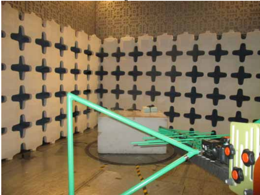
Test Setup for Radiated Emissions – 30MHz to 1GHz, Horizontal Polarization Taoglas Combo Antenna
