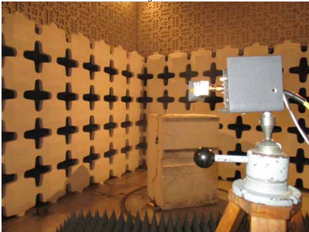
Test Setup for Radiated Emissions – 18GHz to 26.5GHz, Horizontal Polarization Linx Whip Antenna
