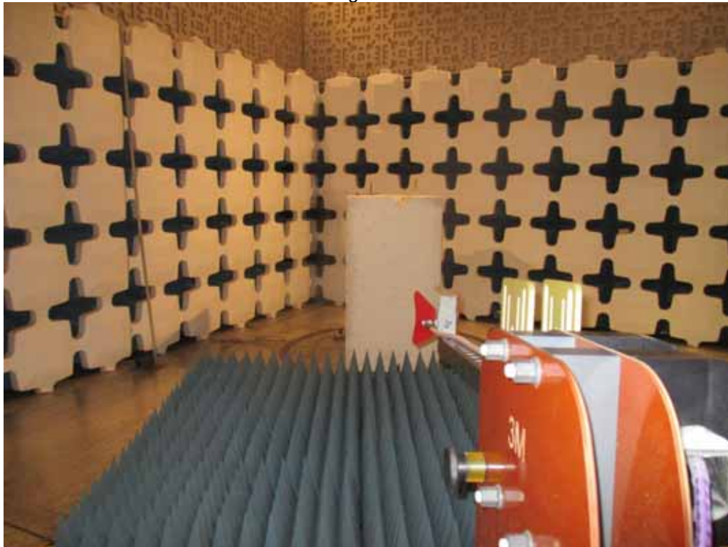
Test Setup for Radiated Emissions – 1GHz to 18GHz, Horizontal Polarization Linx Whip Antenna
