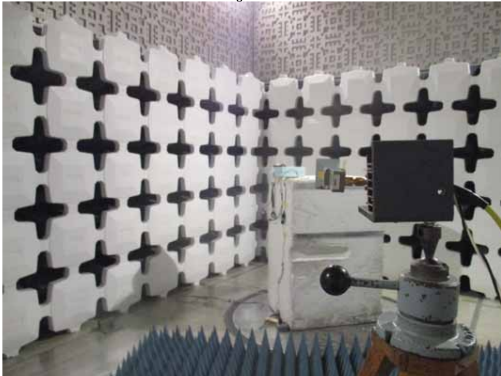
Test Setup for Radiated Emissions – 18GHz to 26.5GHz, Horizontal Polarization Taoglas Combo Antenna
