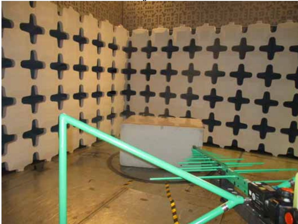
Test Setup for Radiated Emissions – 30MHz to 1GHz, Horizontal Polarization Linx Whip Antenna
