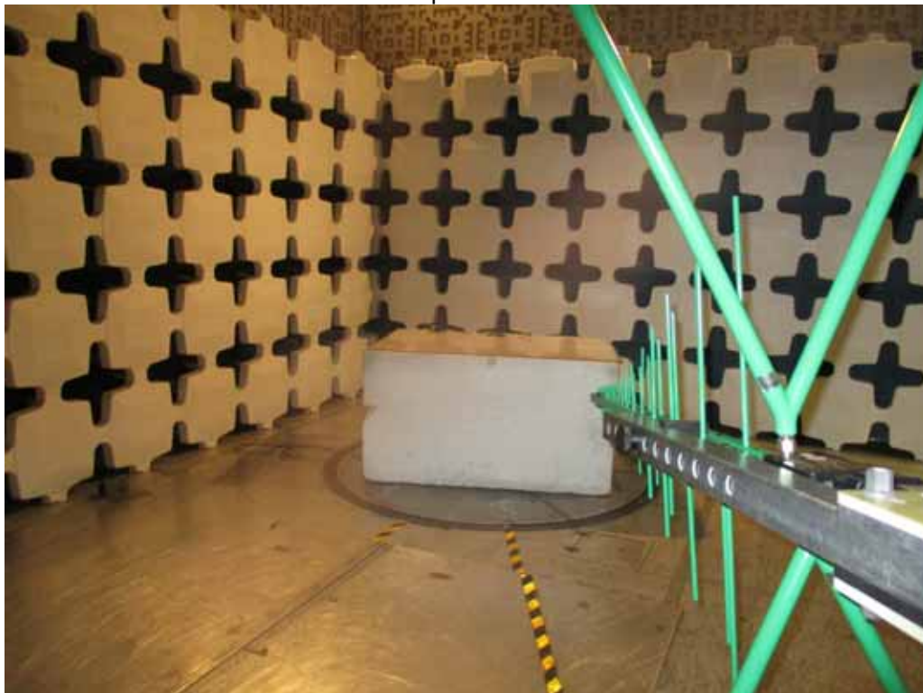
Test Setup for Radiated Emissions – 30MHz to 1GHz, Vertical Polarization Linx Whip Antenna
