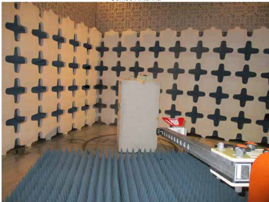
Test Setup for Radiated Emissions – 1GHz to 18GHz, Vertical Polarization Taoglas Combo Antenna
