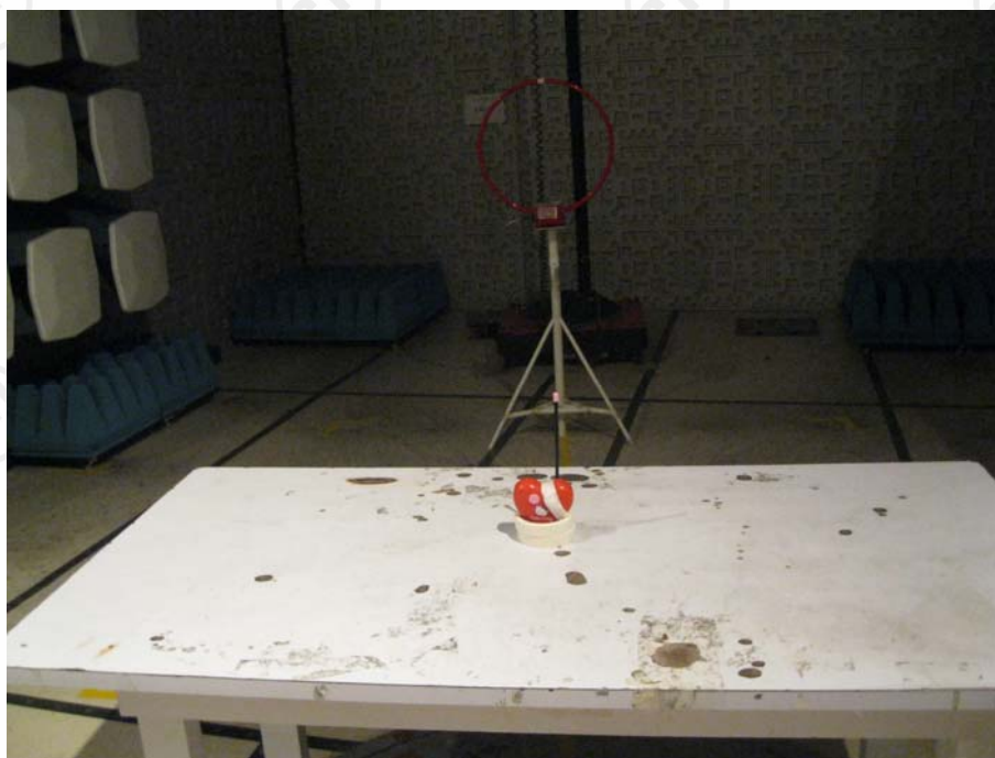
TEST SETUP OF RADIATED EMISSION (9kHz-30MHz)
