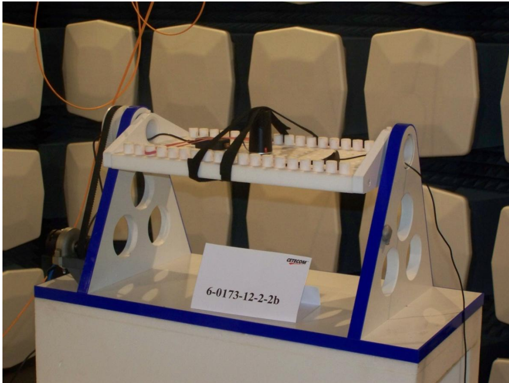
Radiated field strength measurements in the FAR (Fully-Anechoic-Chamber), test setup 1 The letter shall be 'c' at the end instead of 'b'.
