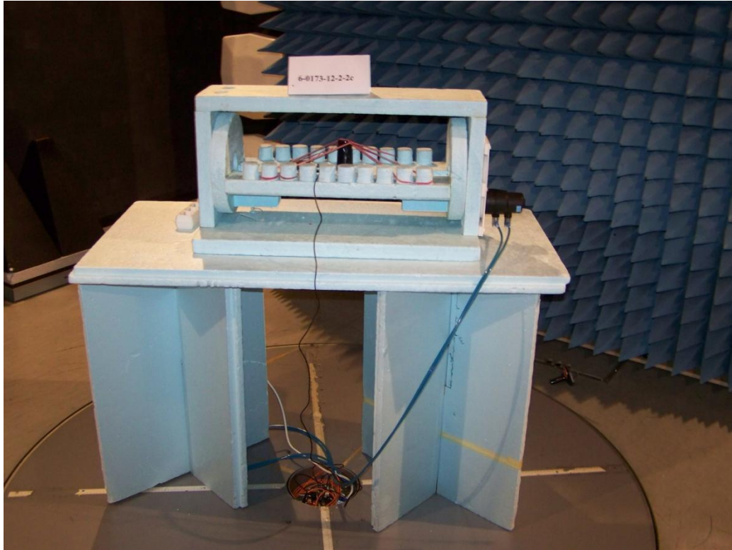
Magnetic field strength measurements in the SAR (Semi-Anechoic-Chamber), test setup 1
