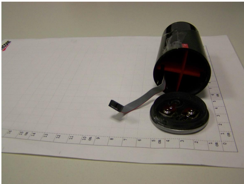
EUT A inside view (space for four batteries type 1.5 V - AA)
