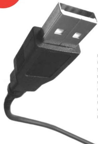
Plug one end of the USB cable into your scale and the other into your computer, which will provide power for the scale and transfer the weight to the Stamps.com software or website automatically. If you do not want to plug the USB cable into your computer you may also use the supplied USB power adapter.
