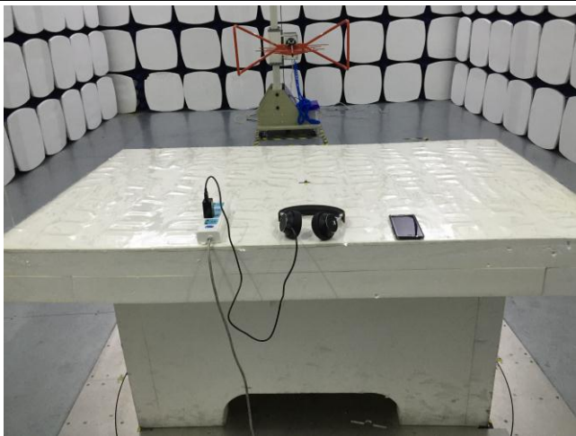
Conducted Emissions Test Setup Front View
