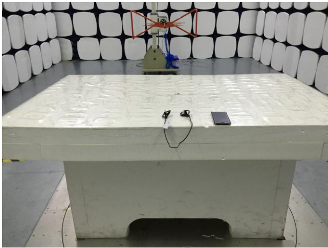
Radiated Spurious Emissions Test Setup Below 1GHz
