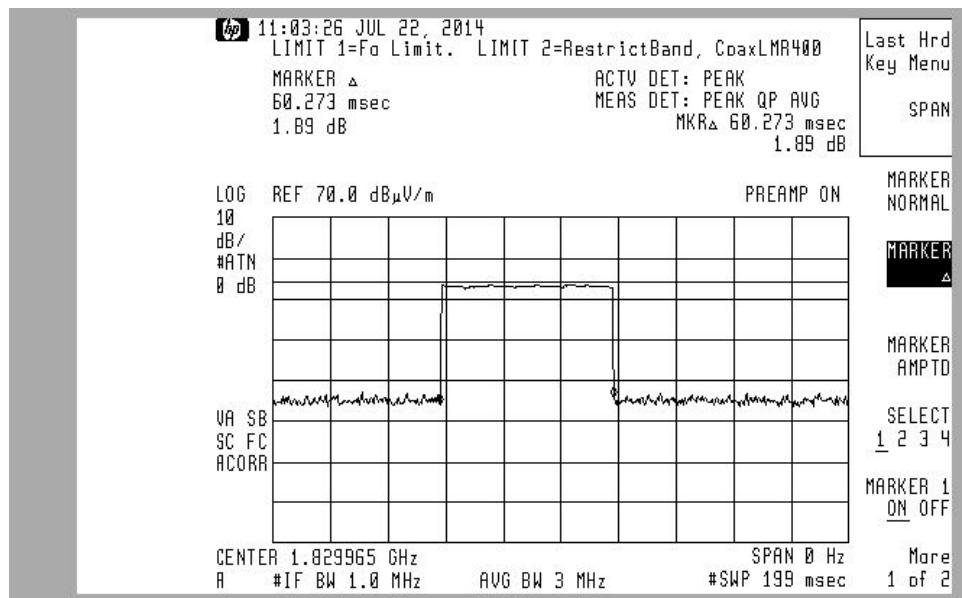
Note: Transmit was measured to be “on” 60 mS out of any 100 mSec period. 60% duty cycle = -4.4 dB correction for averaging peaked harmonic measurements over 1 GHz.
