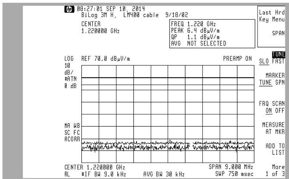
Note: Noise floor only data was recorded at the receiver specified local oscillator frequencies of 305 and 1220 MHz and all associated harmonic measurements.
