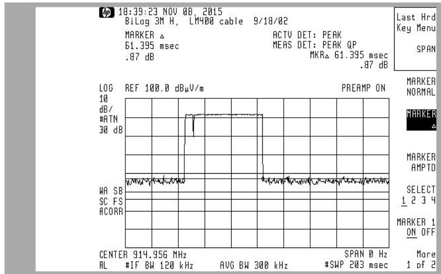
Note: Transmit was measured to be “on” 61.39 mS out of any 100 mSec period. 61.39% duty cycle = -4.24 dB correction for averaging peaked harmonic measurements over 1 GHz.
