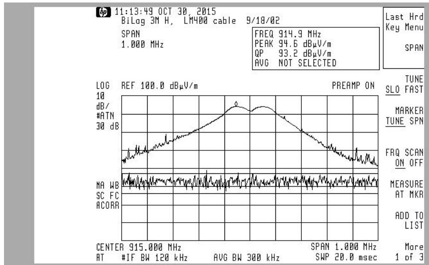
**Transmit Fundamental Measurement**
