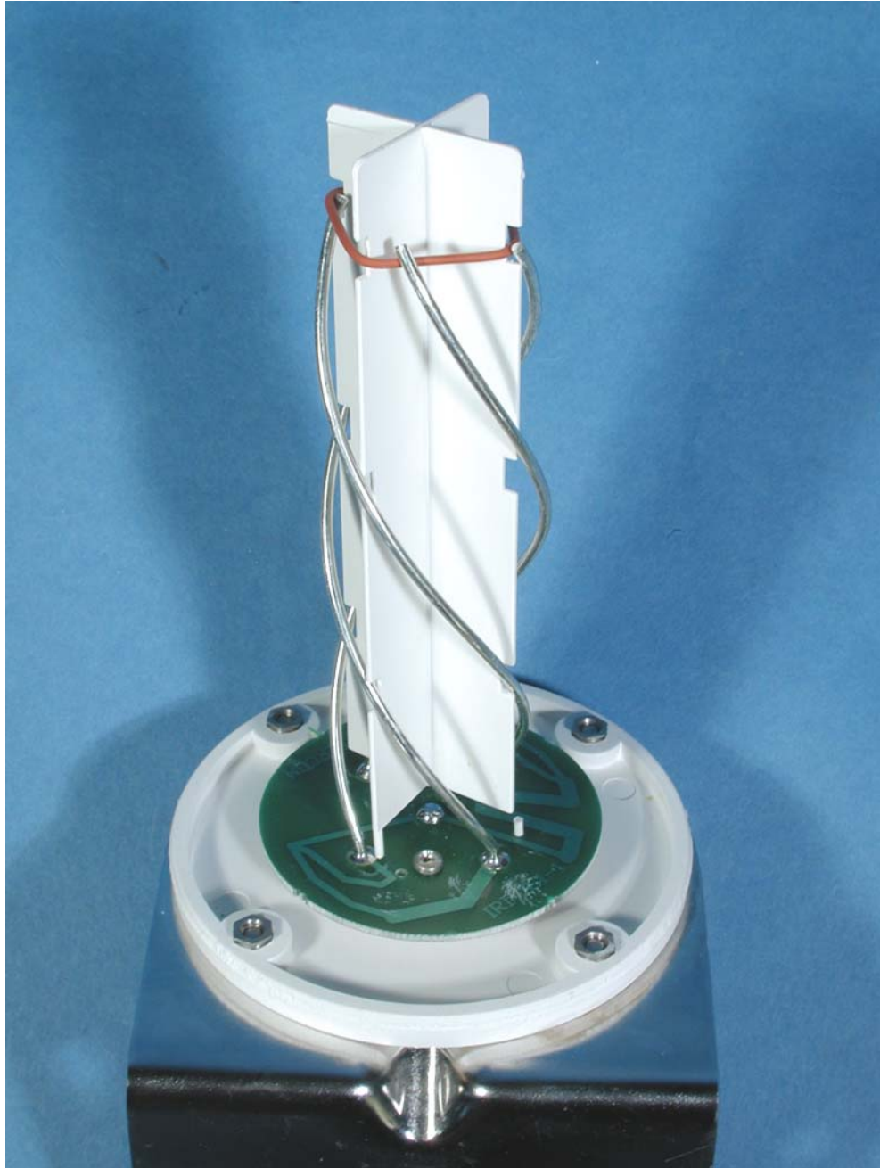
Internal of antenna unit
