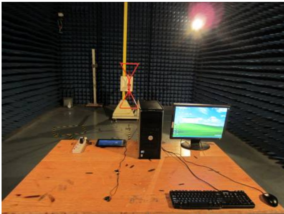
RE TEST SETUP
