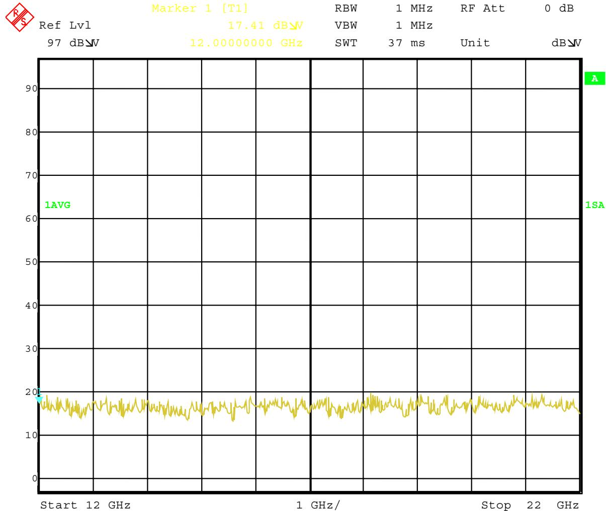
**Channel 660 (this is valid for all 3 channels and up to 20 GHz)****Idle-Mode**
