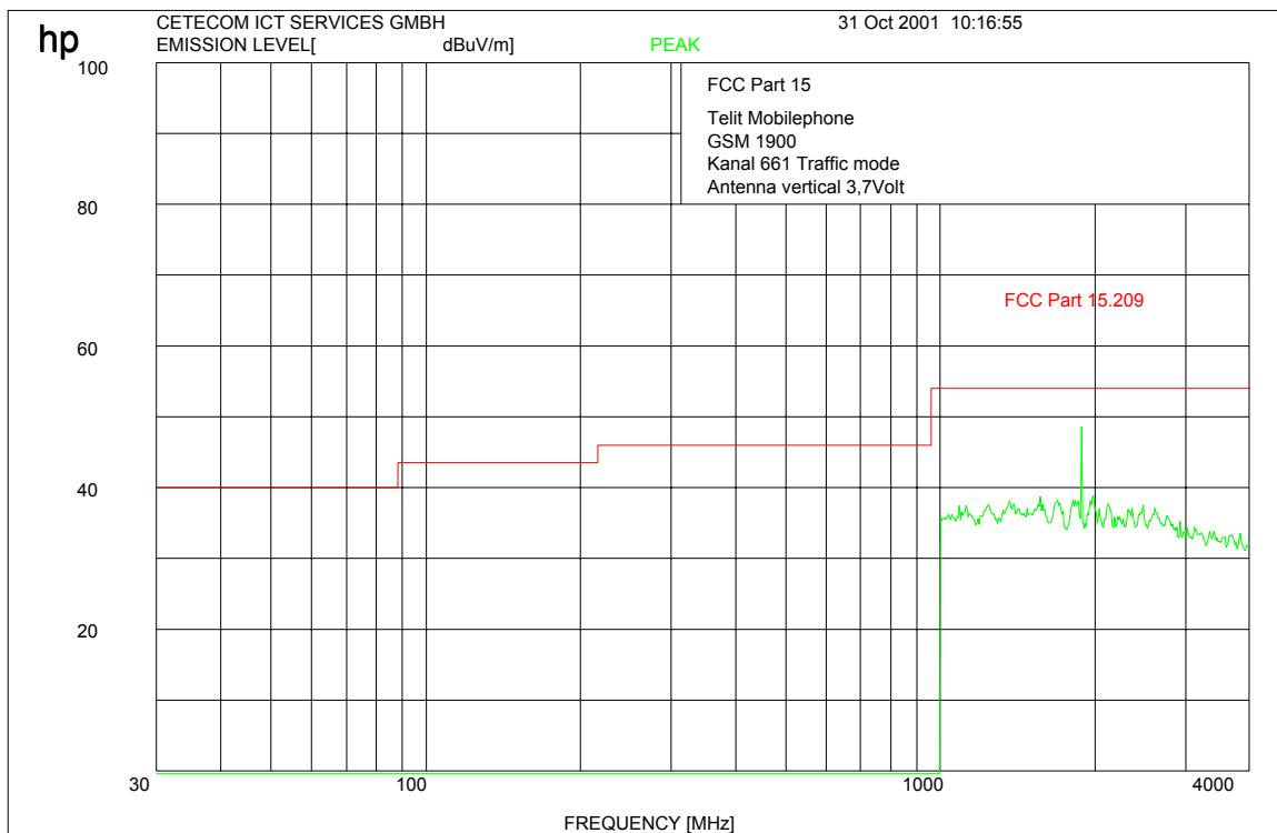
**Carrier is notched with a Band Reject Filter****REFERENCE NUMBER(S) OF TEST EQUIPMENT USED**
