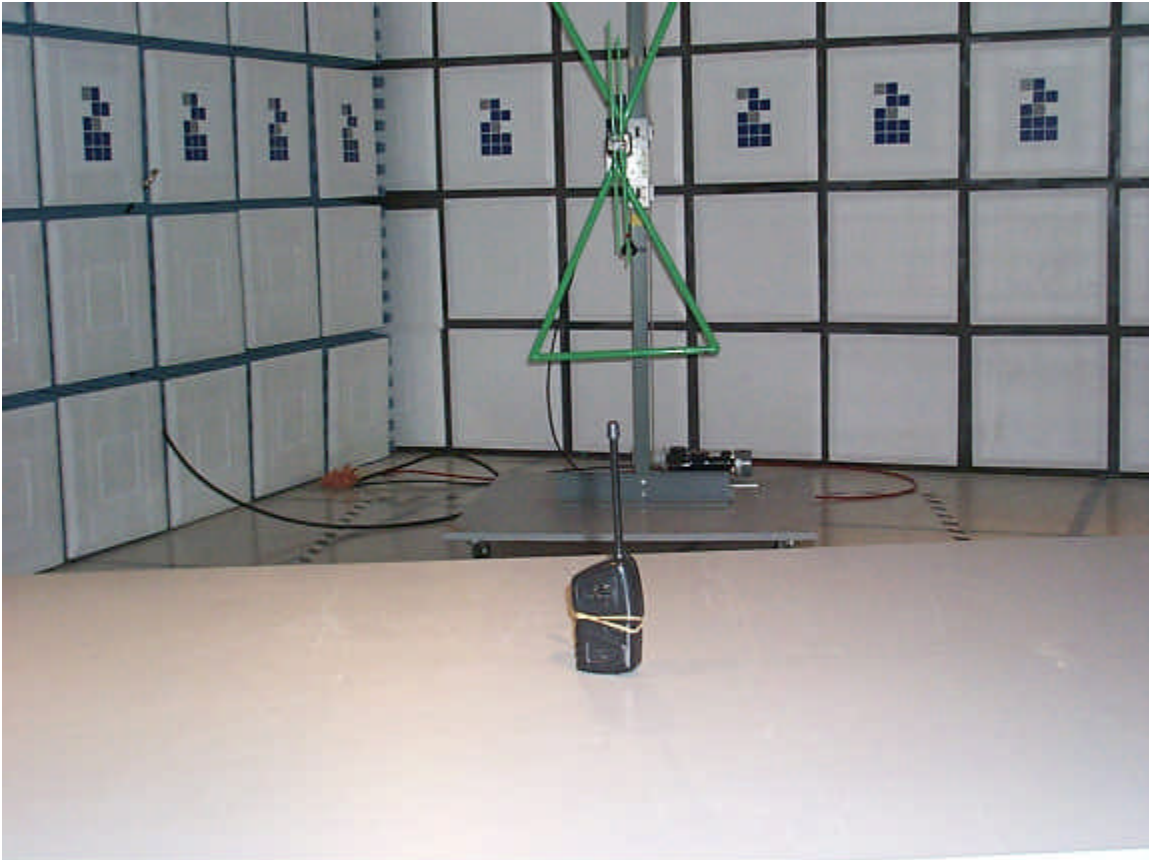
Maximized Radiated Emission Test Set-up – Front View - Vertical
