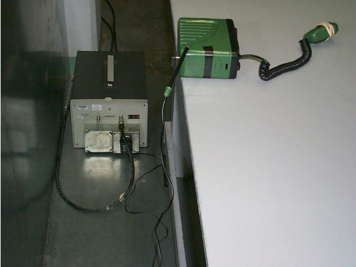
Maximized Conducted Emission Test Set-up - Rear View
