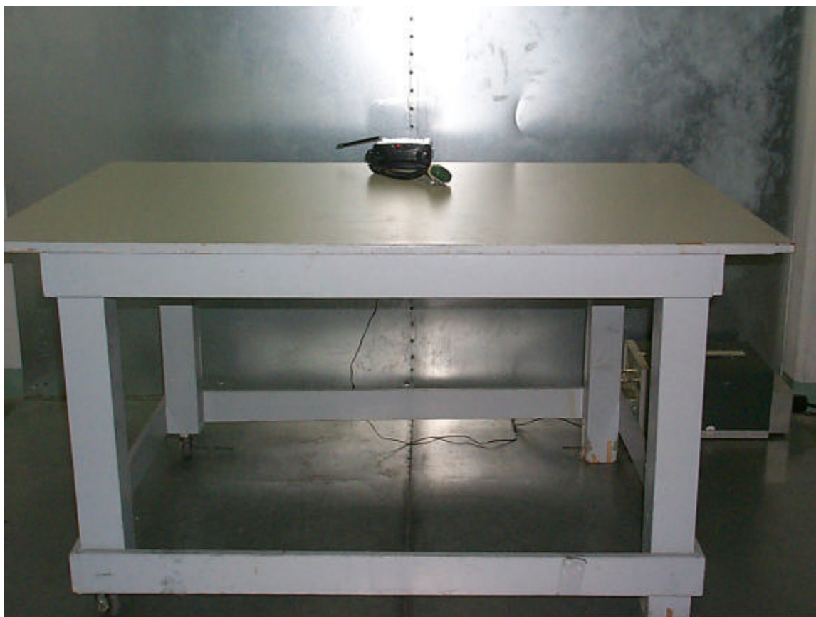
Maximized Conducted Emission Test Set-up - Front View
