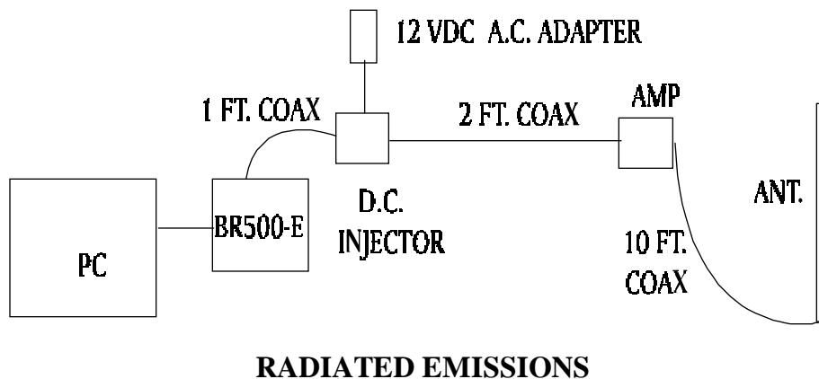
The EUT was set up on the center of the test table, in a manner which follows the general guidelines of ANSI C63.4, Section 6 "**General Operating Conditions and Configurations**". Two sets of measurements were taken: First set with amplifier, second set without amplifier.
