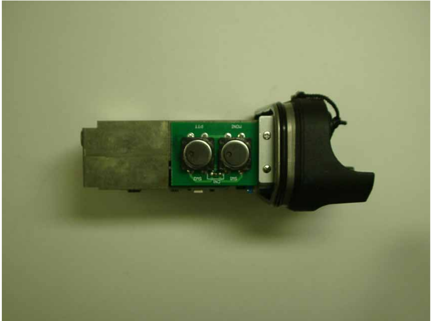
PTT Buttons installed
