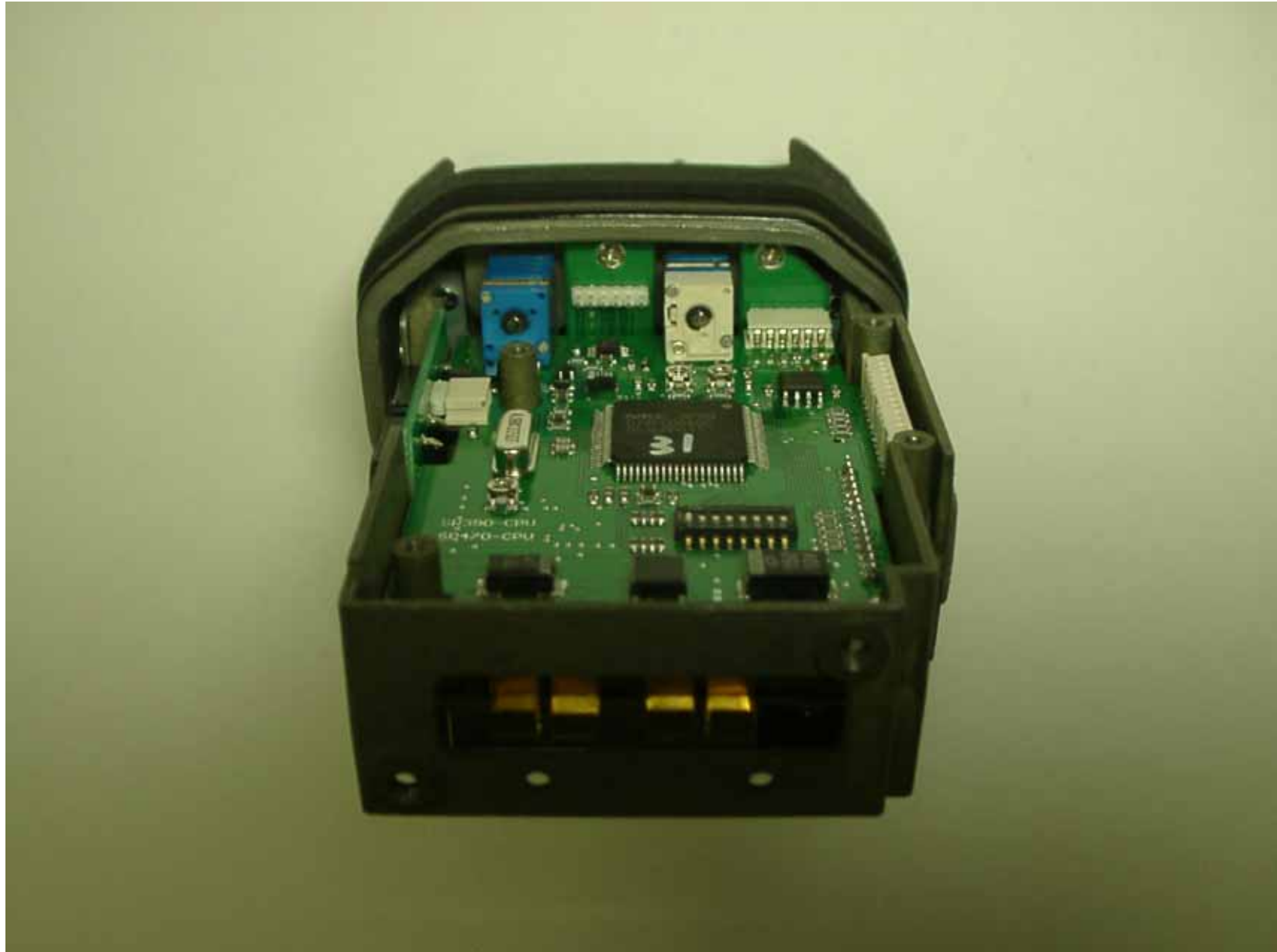
CPU Board installed
