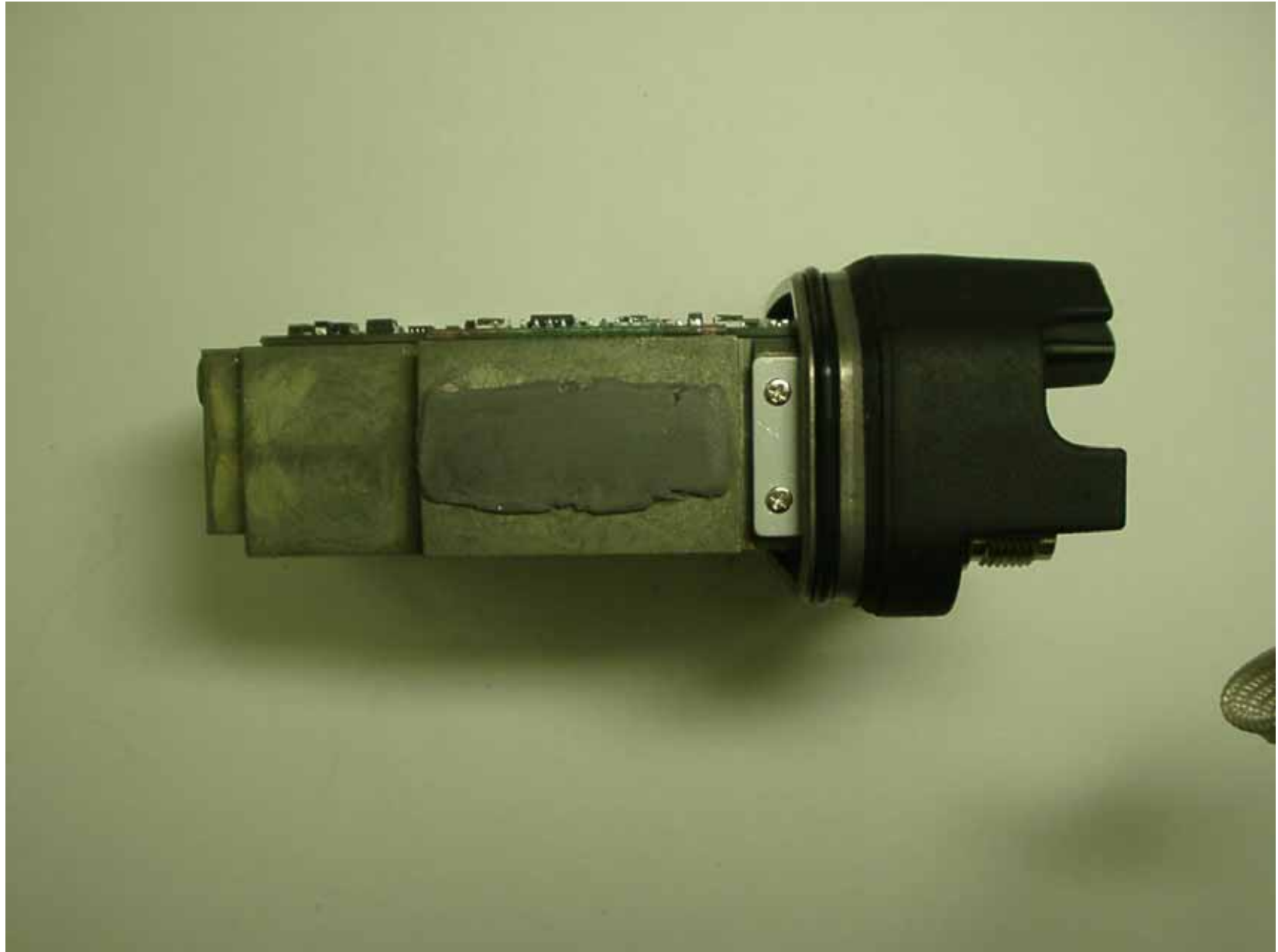
Opposite view of PTT Buttons installed
