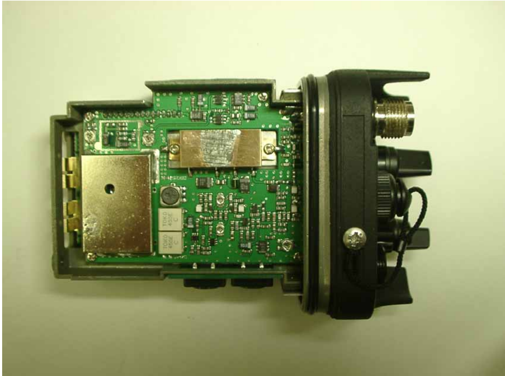
RF Unit with shield removed
