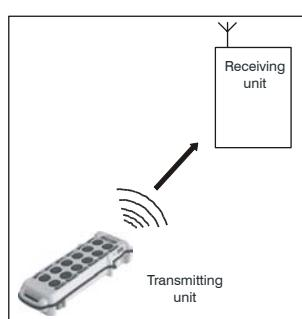
The transmitting unit uses radio frequencies to transmit a coded message which contains a value called address. Each receiving unit can only decode the messages coming from a transmitting unit with the same address.
