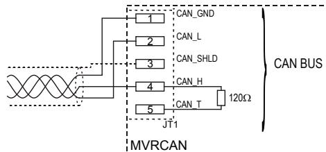
Both ends of CAN networks must be terminated with a 120 Ω resistor between CAN\_H and CAN\_L.
