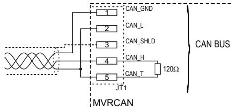
All CAN network nodes must have the same bit rate. The bit rate defines the maximum length for the network:
