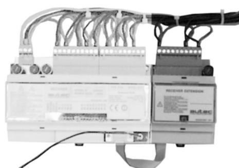
Inside the (receiver) extension unit one of the E16RI\_\_ interfaces may be mounted (see the different Configurations)
