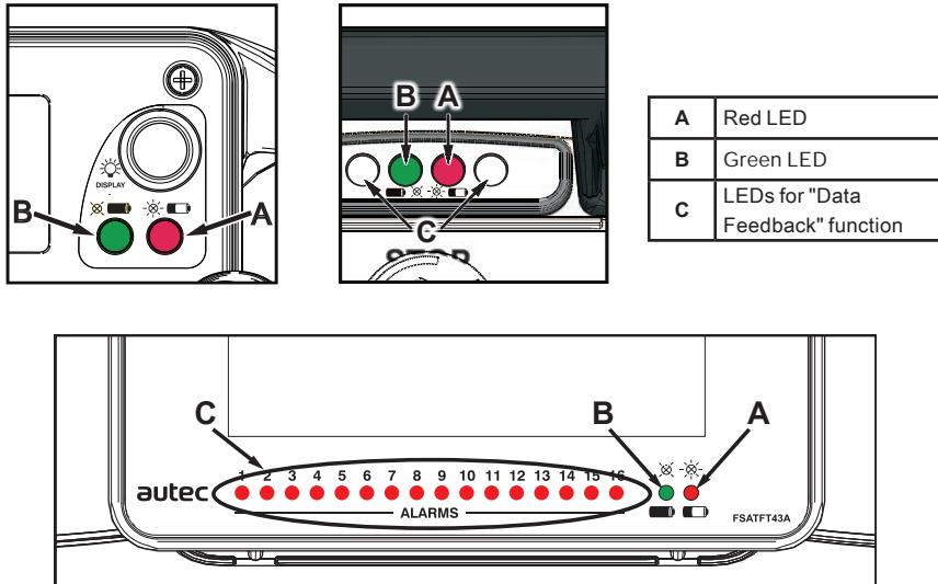
The Transmitting Unit always has a green LED [B] and a red LED [A] that provide information regarding the Radio Remote Control.
