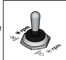
This switch increases (rpm +) or decreases (rpm -) the number of revolutions of a Machine's engine.
