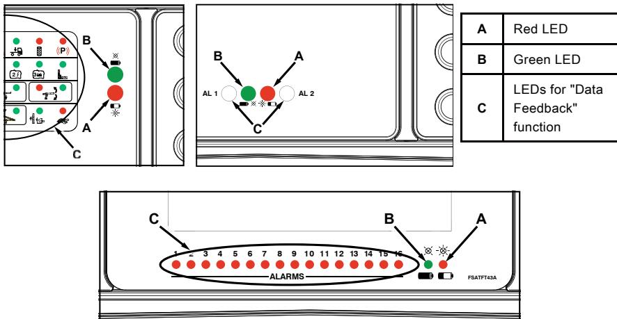
The FJB Transmitting Unit always has a green LED [B] and a red LED [A] that provide information regarding the Radio Remote Control.
