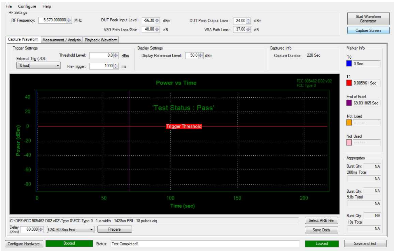
Figure 8.9-1: Radar burst at the end of the CAC
