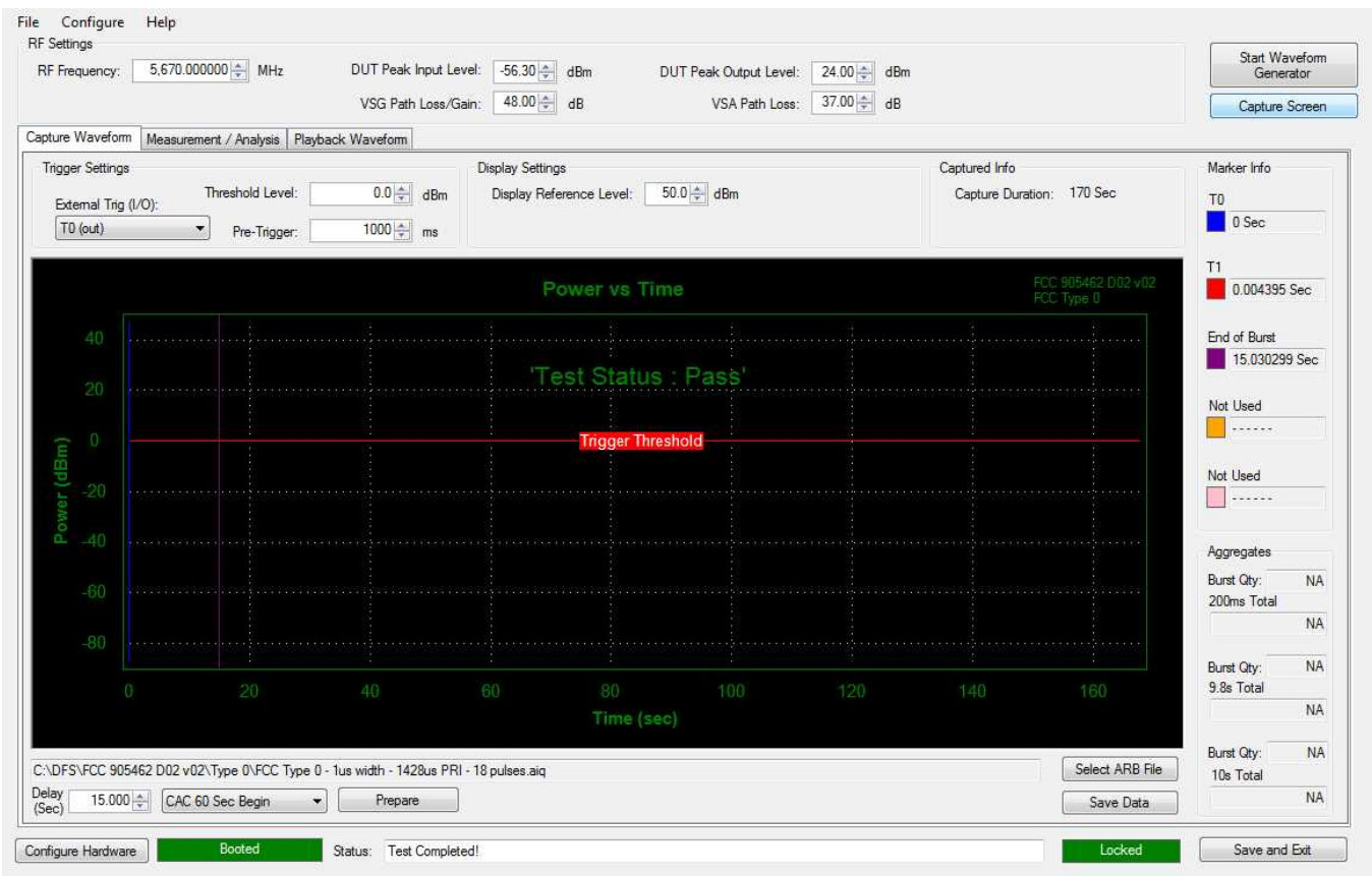
Figure 8.8-1: Radar burst at the beginning of the CAC
