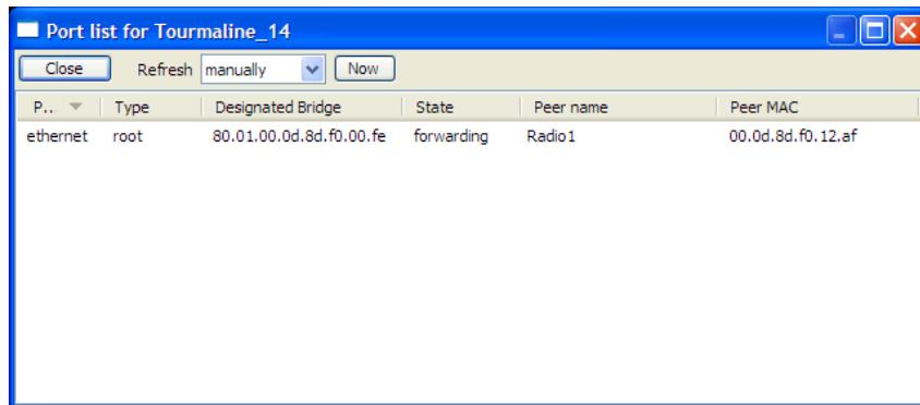
The port table is a list of all the active ports on the radio. This list shows the same information as the Port status (page 56) list in the Radio Configuration / Diagnostic Utility. Each radio can have up to 34 active ports—one Ethernet cable, one parent RF link, and up to 32 child RF links.
