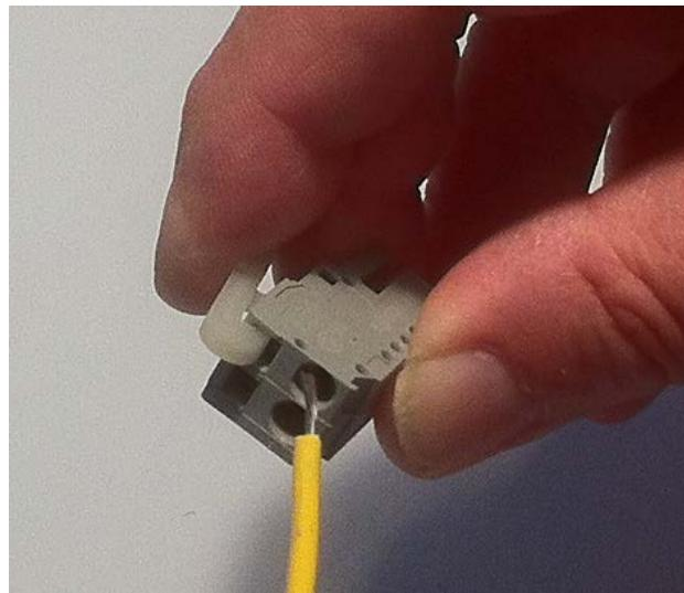
Press down on the installation tool to use it as a lever which will open the connector's contacts to insert a wire. A properly-wired power connector is shown:
