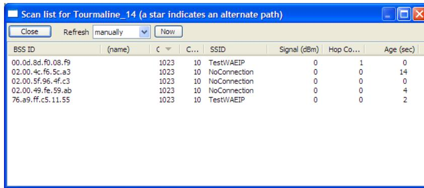
The scan list is a list of all the radios that this particular radio "hears" on this channel (via beacons) even if it is not linked to it (different SSID or encryption). This list shows the same information as the Available Parents list in the Radio Configuration / Diagnostic Utility.
