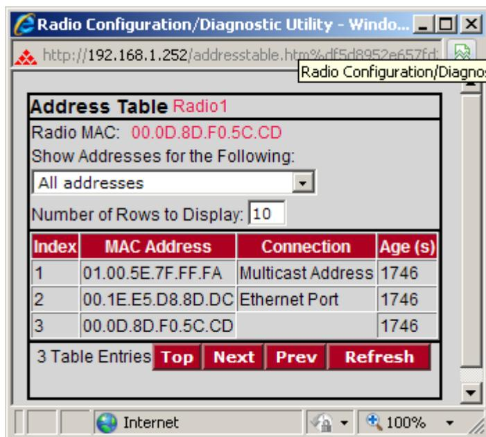
The Address Table shows the port through which each MAC address is connected, along with the age in seconds since the radio last saw a packet from this MAC address.
