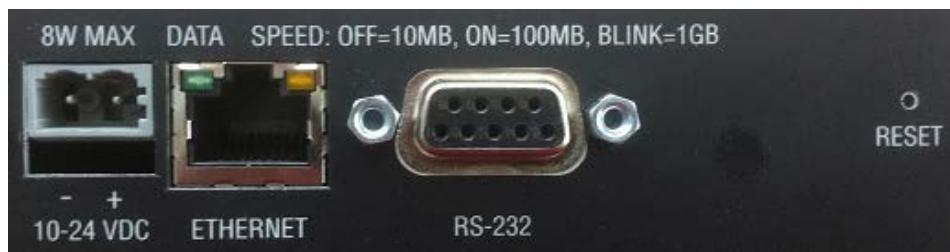
1. Attach an Ethernet cable to the designated master RLX2 radio. Make sure this network connection is on the same subnet as the PC running the IH Browser configuration software.
