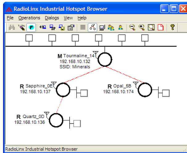
The Topology view shows a diagram of the network's wireless connections. Use this view to see whether all the radios are linked, and approve of the way the radios are linked.
