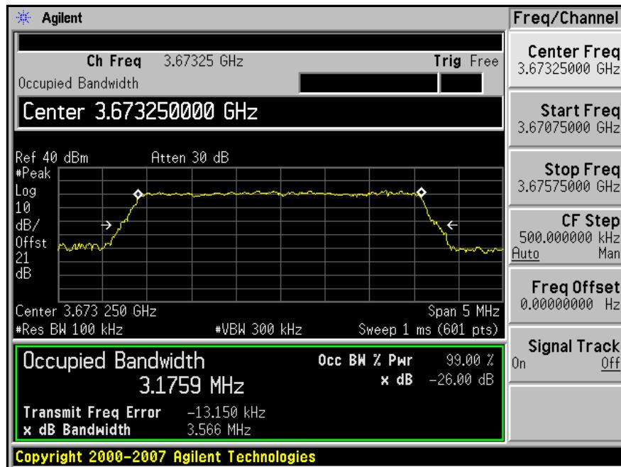
**Channel Bandwidth = 7.0 MHz****Low Channel (Fc = 3653.50 MHz)**
