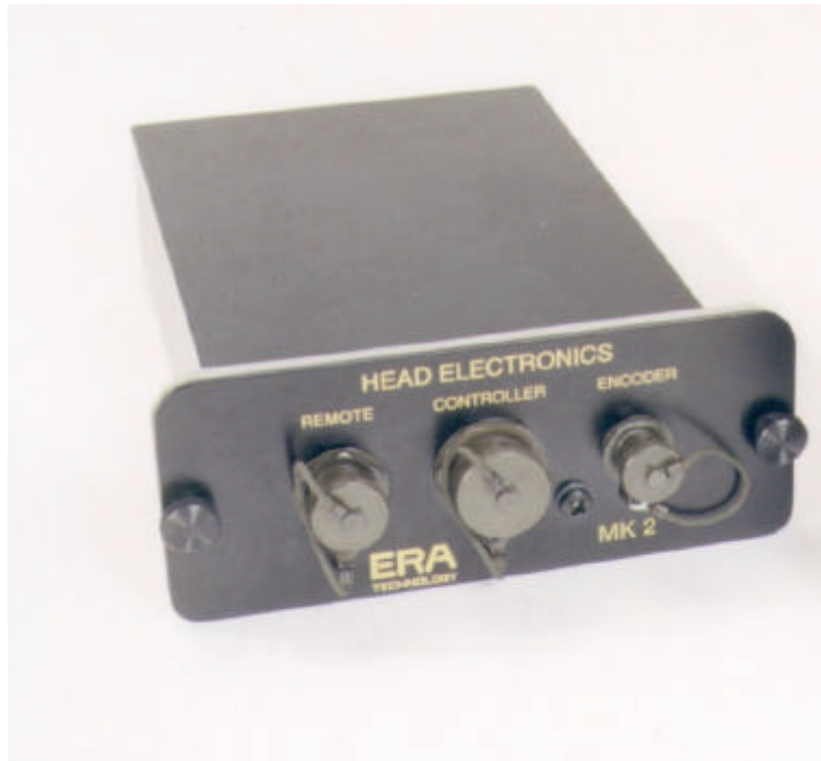
Fig. 13: SPRscan head electronics
