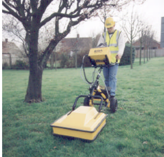
Trolley Mode – with 250 MHz antenna
