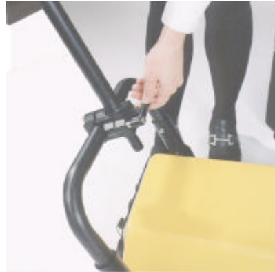
Loosen the locking clamp and straighten antenna so that it lies flat. Tighten up the clamp
