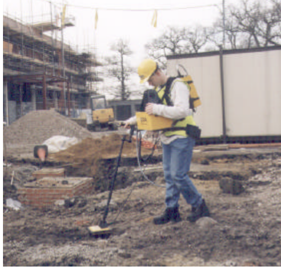
One-man mode – with 1 GHz antenna. The 500 MHz antenna can also be used in this configuration
