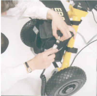
Connect the battery to the controller using the black curly cable
