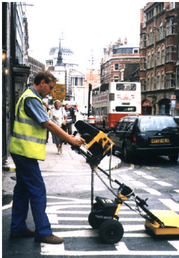
Trolley Mode – with 500 MHz antenna
