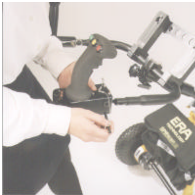
Locate and fix the function handle to the stub. Lock it in place with the PIP pin supplied
