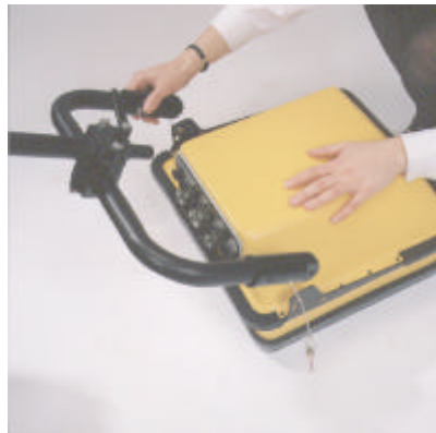
Remove the PIP pins and position the 500 MHz antenna between the clevis
