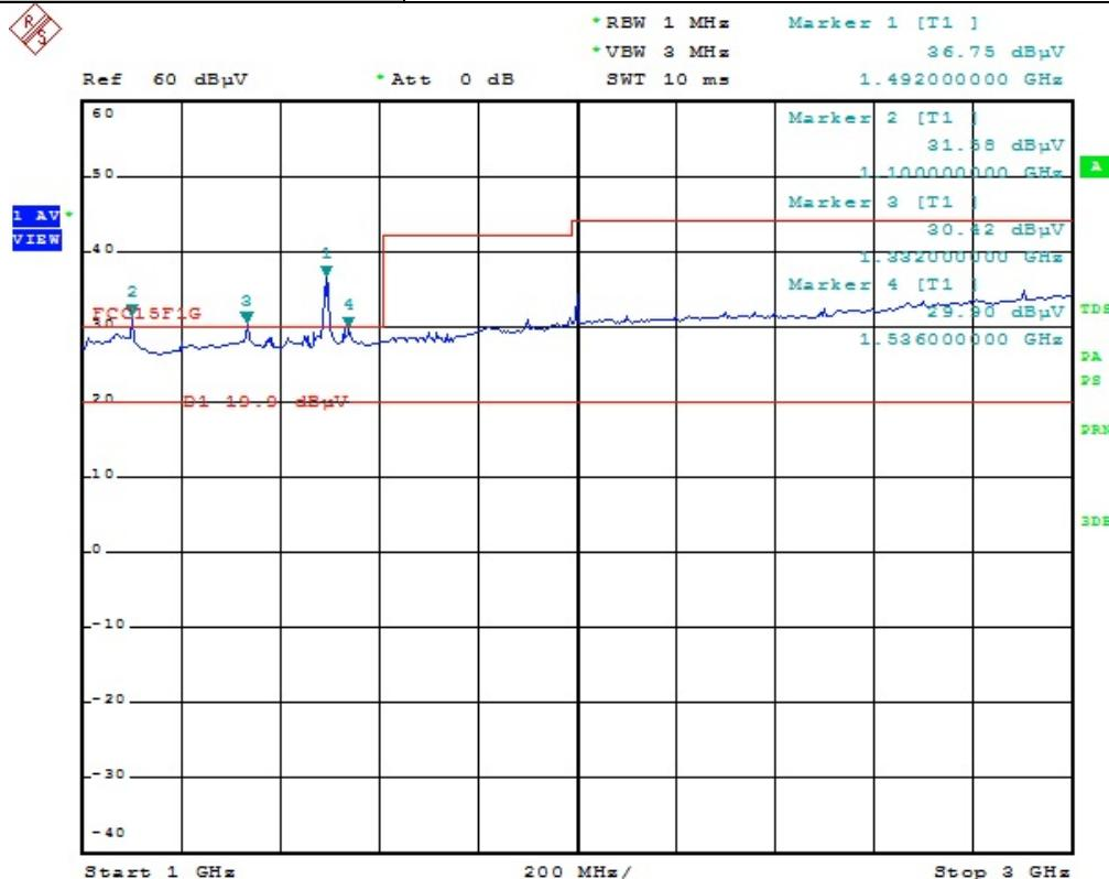
All marked emission points are from Digital Circuitry (see Test No.1) and shall be excluded for FCC Part 15F application.
