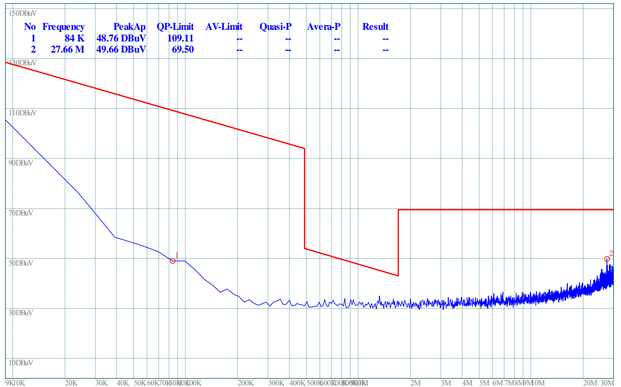
(Plot A.1: 9kHz to 30MHz)
