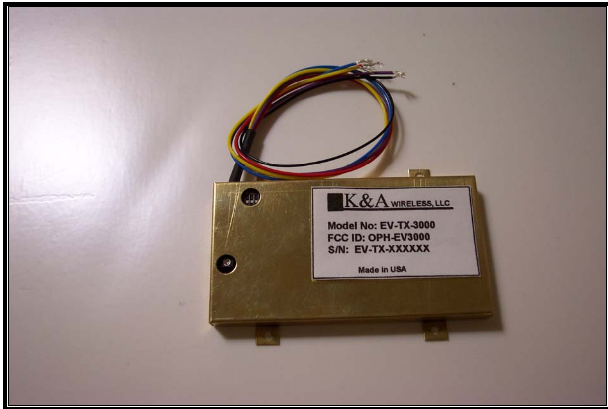
Photograph 3: External Shielding with Label
