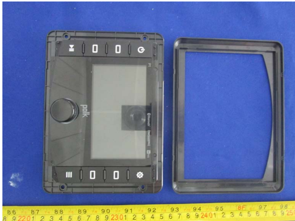
EUT – Controller Panel Uncover View
