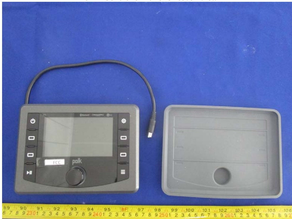
EUT – Controller Panel Uncover View
