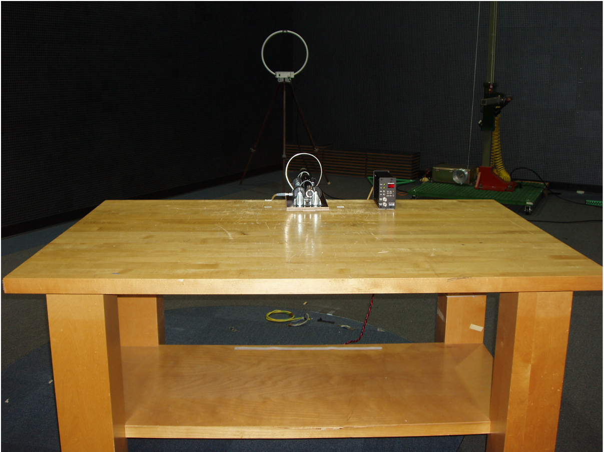
Photo 3 – Rear View of the 5 m Radiated Emissions Test Set-up
