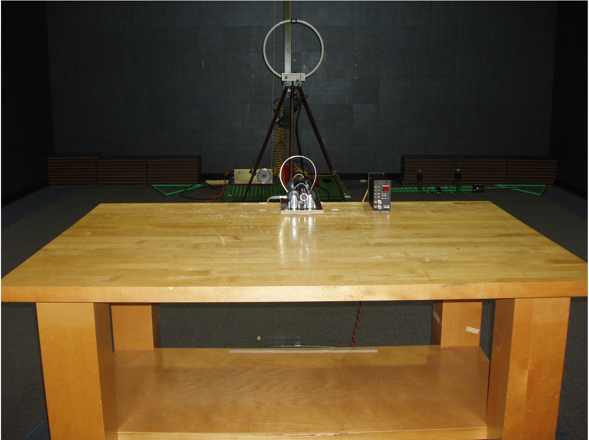
Photo 2 – Rear View of the 3m Radiated Emissions Test Set-up
