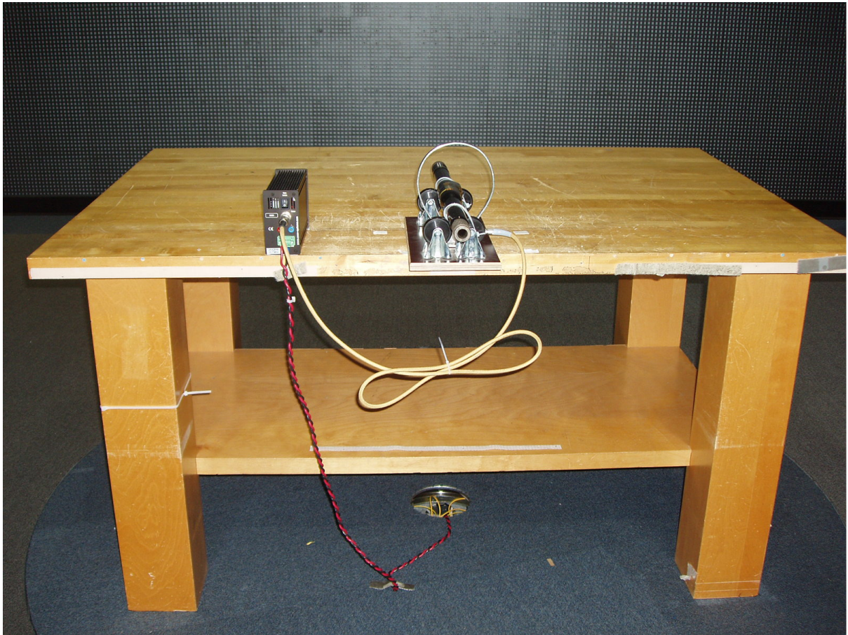
Photo 1 – Front View of the 3 m Radiated Emissions Test Set-up
