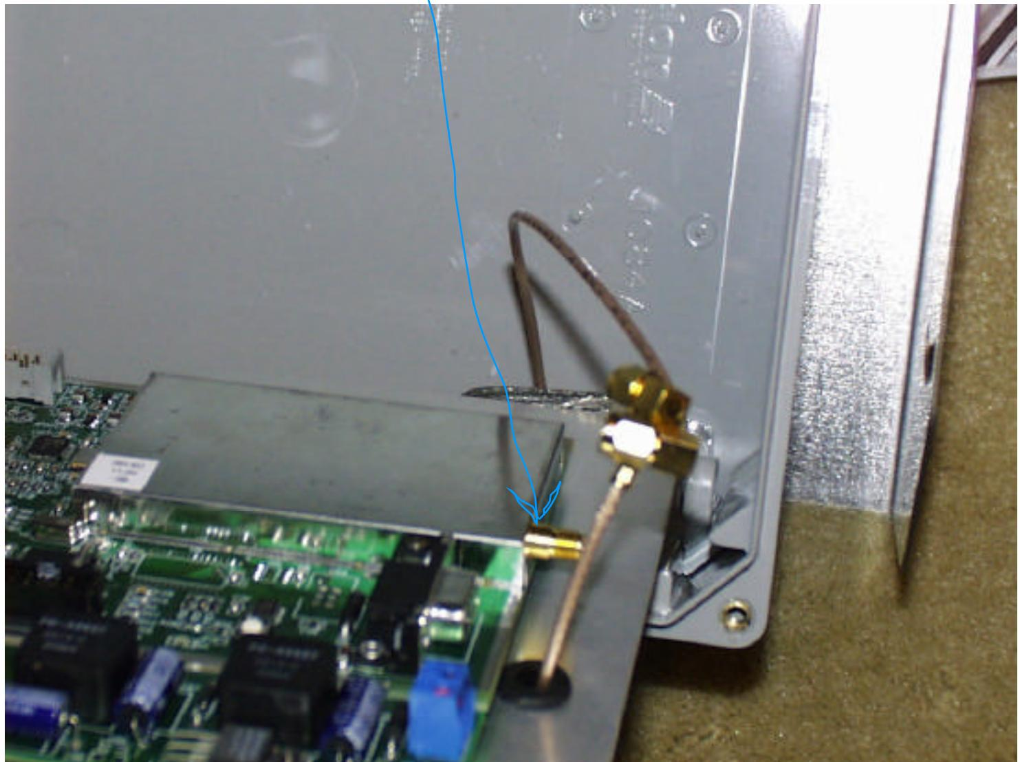
Internal antenna cable connection at interna antenna
