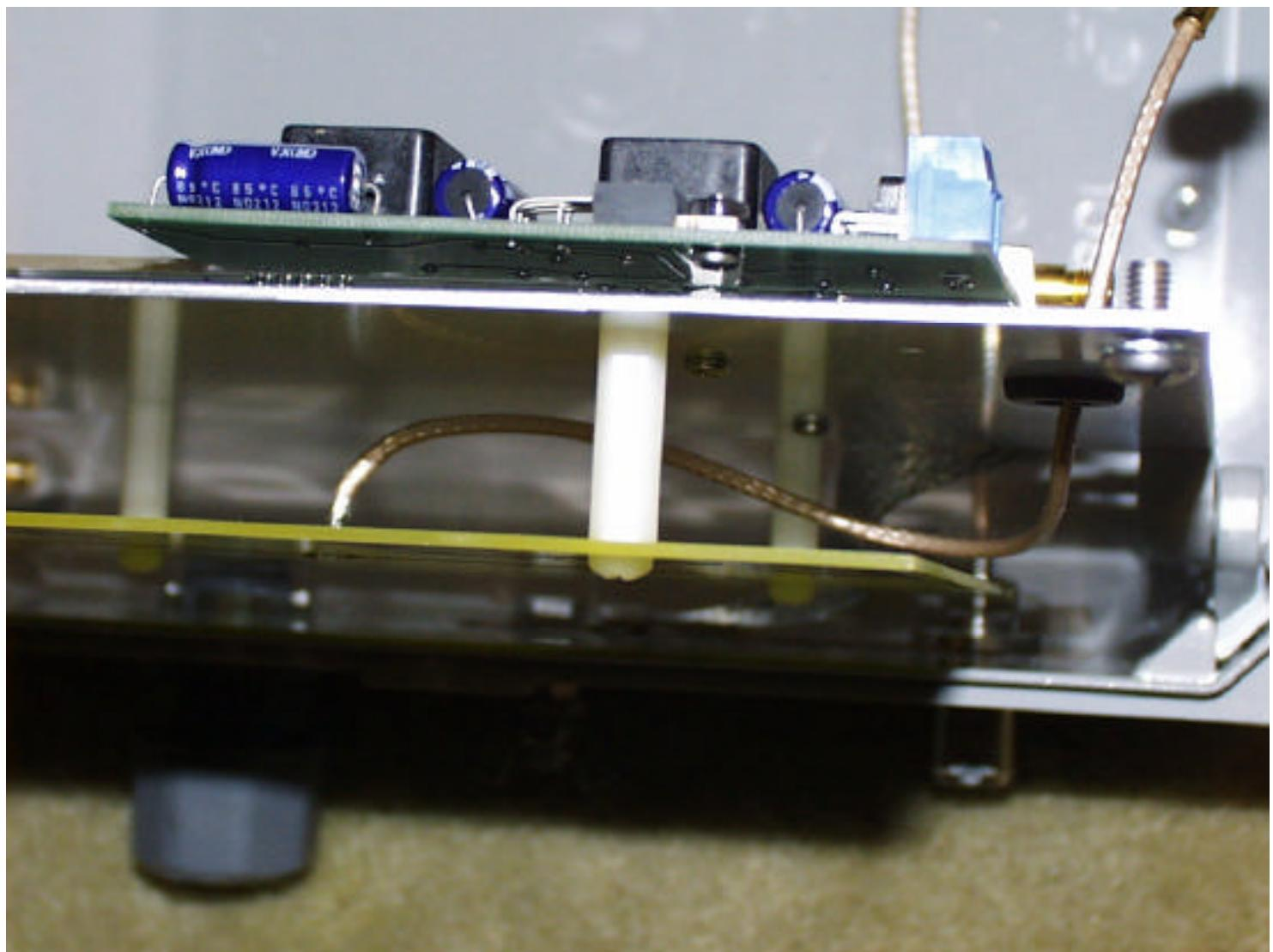
Internal view of reverse SMA cable going to external N connector
