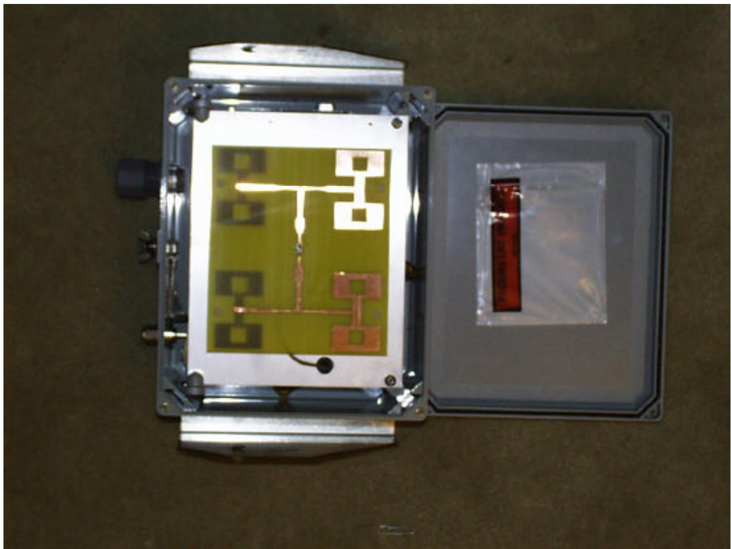
Two cables, one to internal antenna, one to outside N connector
