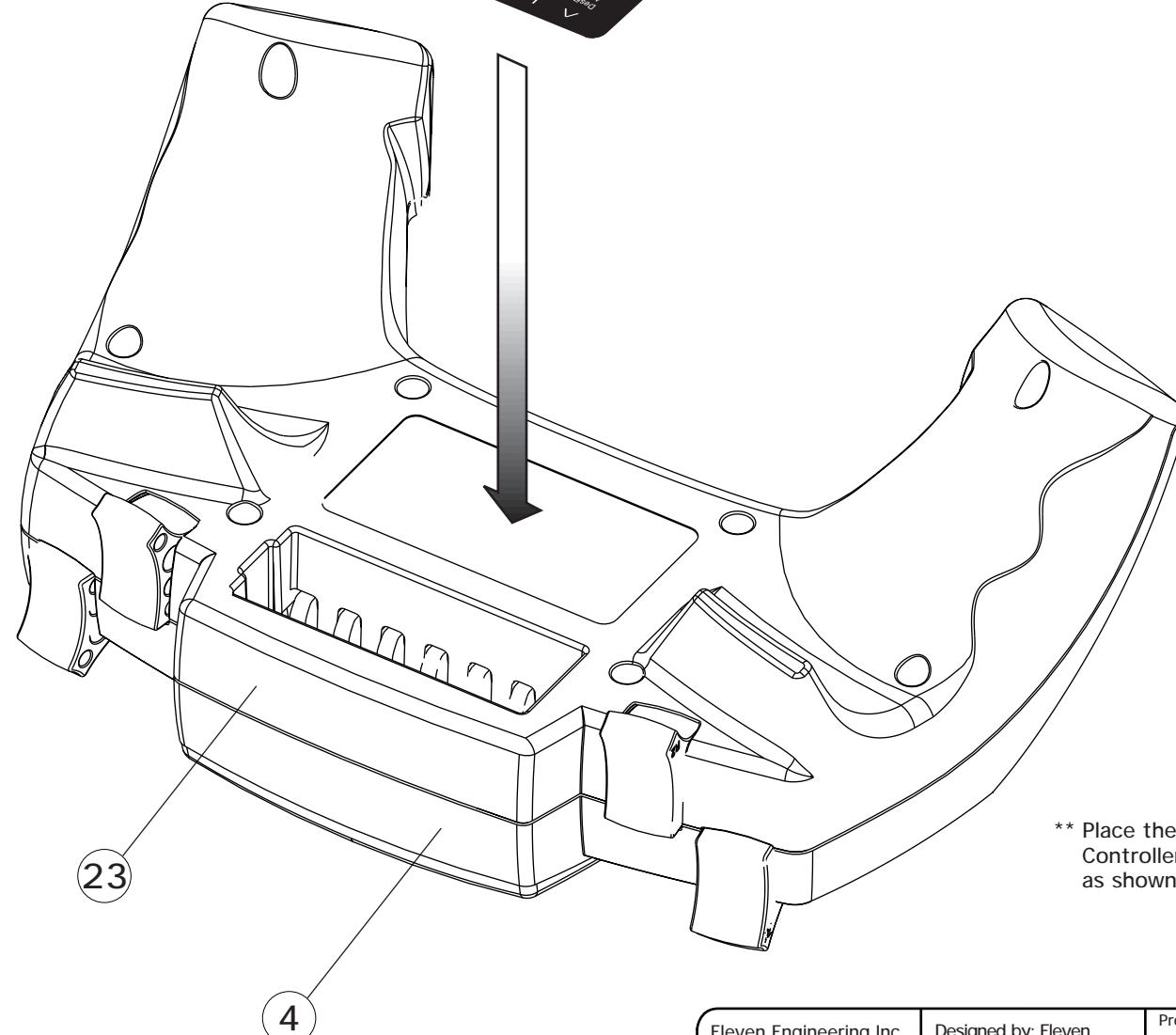
\*\* Place the Sticker(25) onto the Controller Bottom Clamshell(23) as shown.
