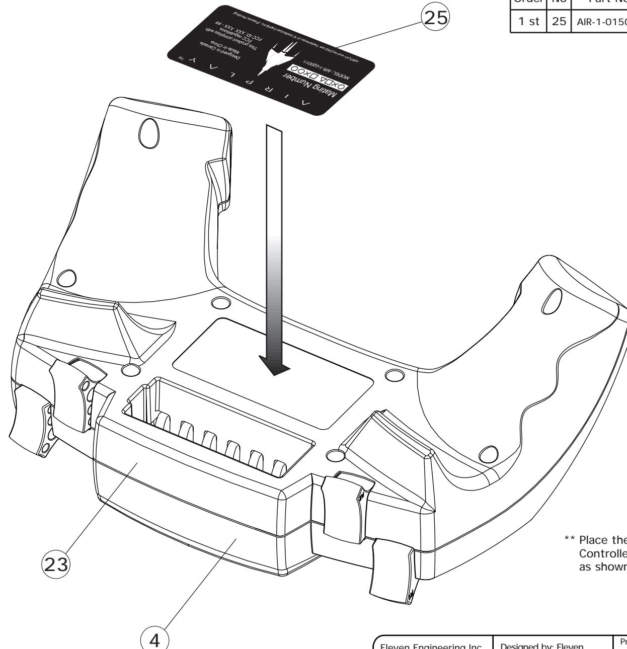
\*\* Place the Sticker(25) onto the Controller Bottom Clamshell(23) as shown.
