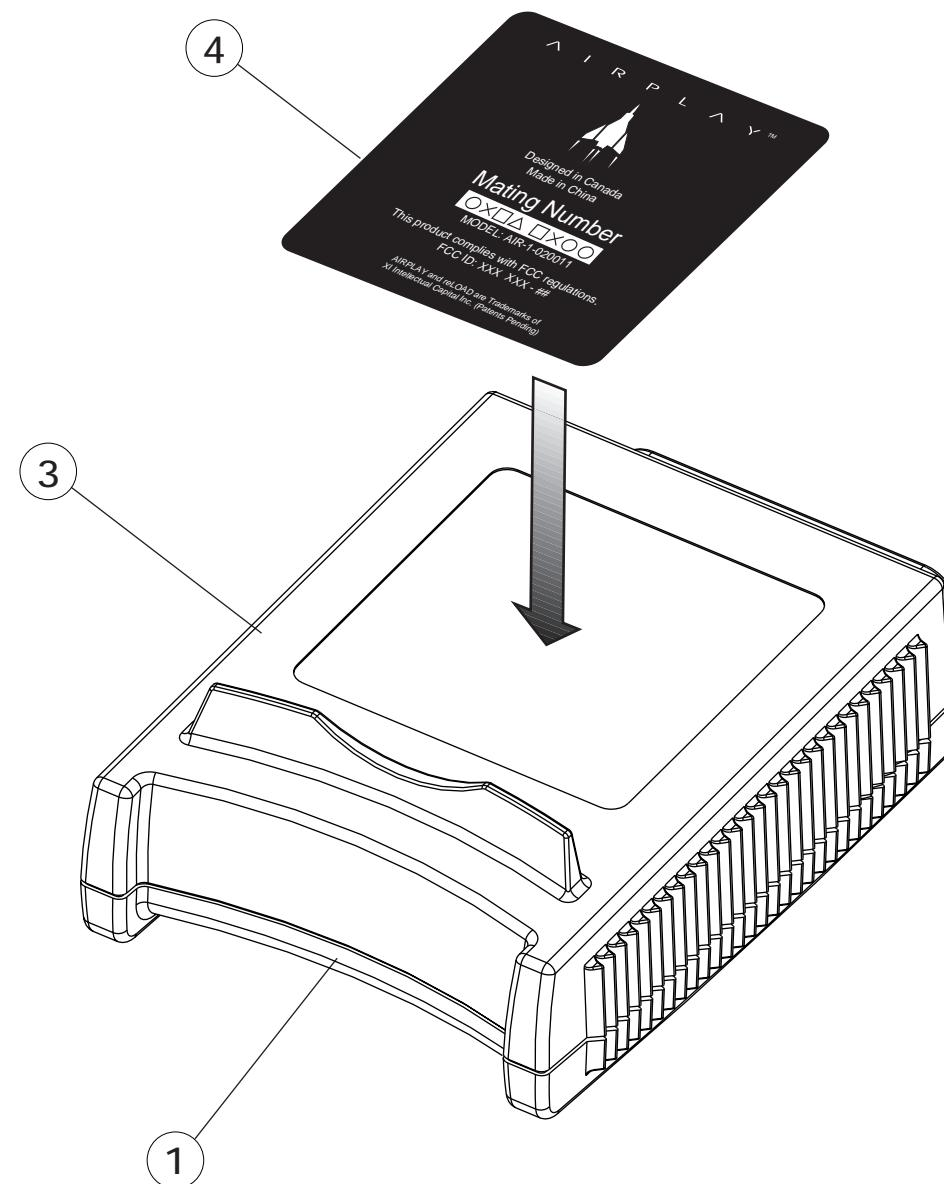
\*\* Place the Sticker(4) onto the Receiver Bottom Clamshell(3) as shown.
