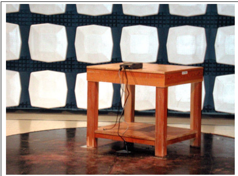
Picture of Radiated Emissions Setup: EUM 3003.
