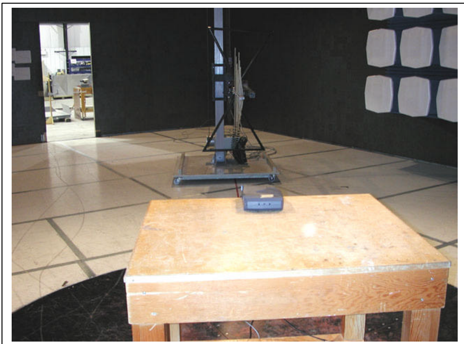
Picture of Radiated Emissions Setup: EUM 3003.
