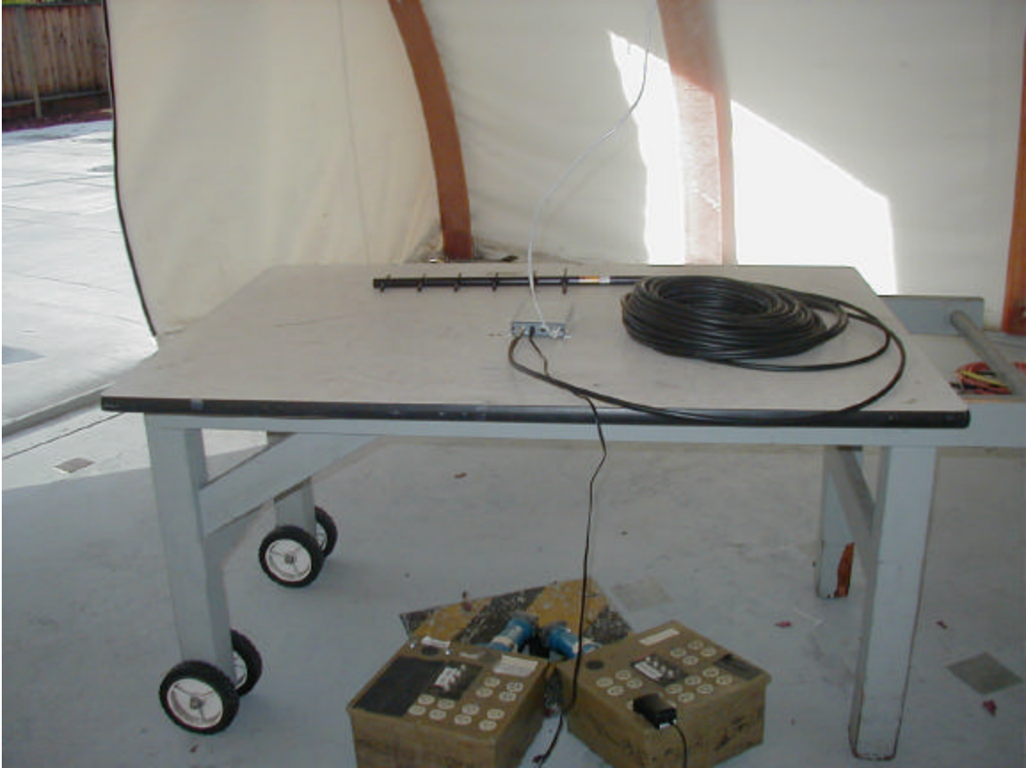
Test Configuration for Radiated Emissions – Yagi Antenna
