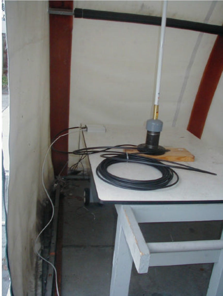
Test Configuration for Conducted Emissions – Side View
