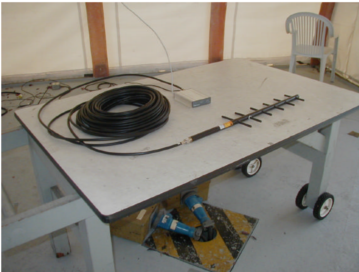
Test Configuration for Radiated Emissions – Yagi Antenna
